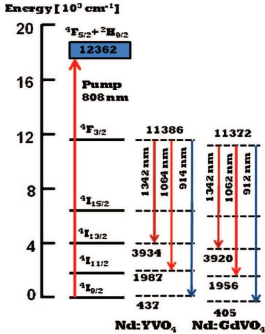
Figure 1. Energy level diagram of Nd<sup>3+</sup>-doped vanadate crystals. The downward arrows represent the major transitions at 1.06, 1.3 and 0.9 μm. The upward arrow represents the pump transition under diode pumping.
