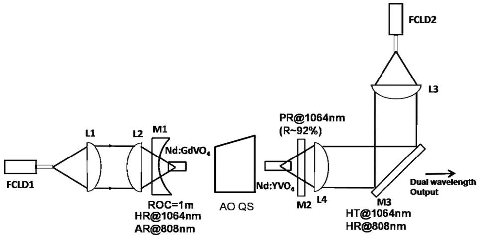
Figure 2. Schematic of the dual wavelength laser set-up.
