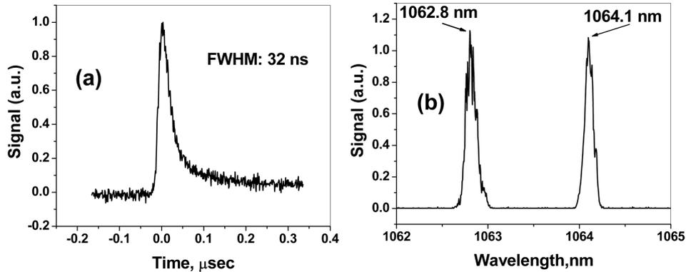
**Figure 4.** (a) Q-switched pulse shape and (b) spectral profile from the hybrid laser.
