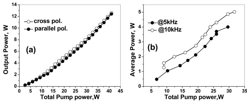
Figure 3. Slope efficiency curves of the hybrid laser. (a) CW operation and (b) pulsed operation.
