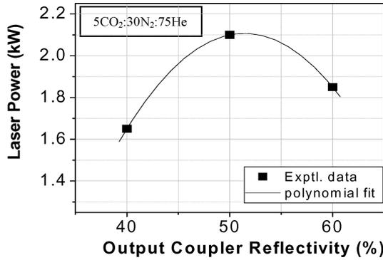
Figure 3. Optimum coupler reflectivity.
