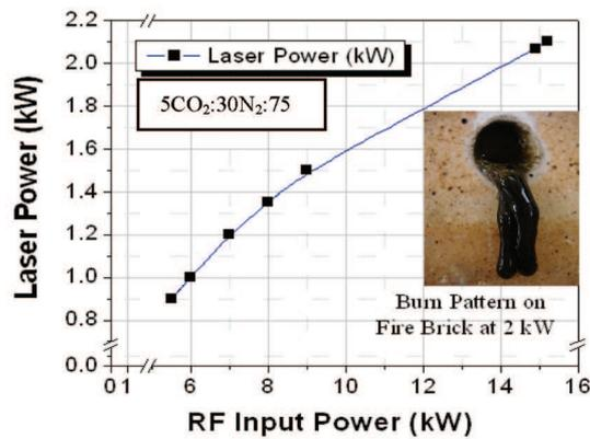
Figure 4. Laser power vs. RF input power (inset) Burn pattern at 2 kW.
