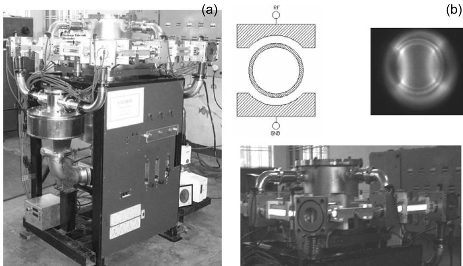
**Figure 1.** (a) RF-FAF CW CO<sub>2</sub> Laser. (b) Electrodes assembly, end-on view of RF glow discharge, simultaneous RF-excitation.
