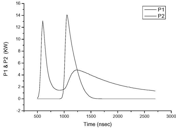
**Figure 1.** Output from rotating mirror Q-switch laser. The time is measured from the instant of q-switching. The first pulse is the  $10.53 \mu\text{m}$  pulse and the second pulse is the  $13.9 \mu\text{m}$  pulse.
