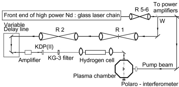
**Figure 1.** Schematic of the SRS probe beam.
