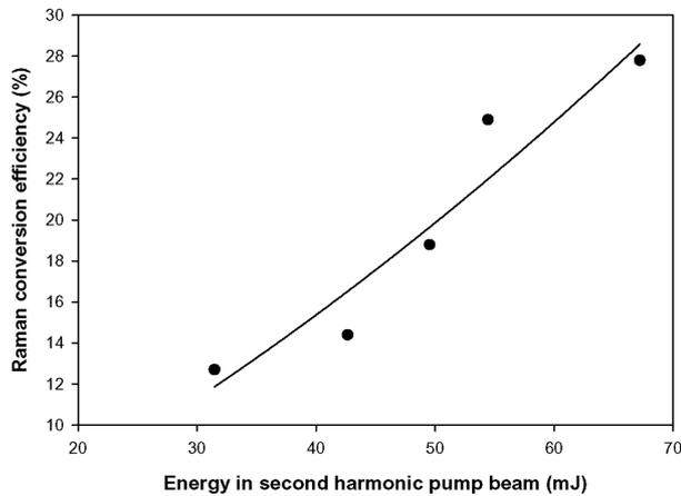
**Figure 2.** Conversion efficiency of hydrogen SRS cell.
