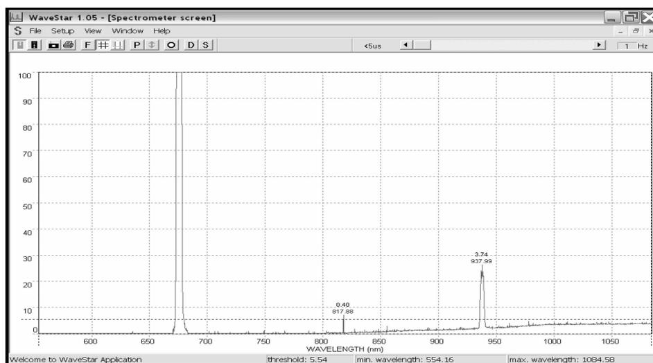
**Figure 3.** Stokes spectrum of hydrogen showing the first Stokes wavelength at 673.75 nm and the second at 937.99 nm.
