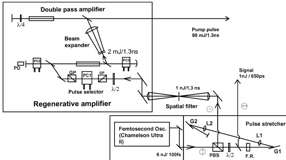
Figure 1. Experimental scheme for the generation of pump and signal laser pulses.
