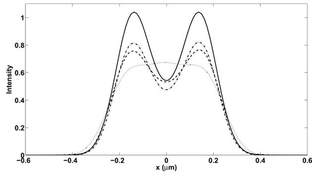
**Figure 8.** Same as figure 7b but with the NIM slab impedance-matched to free space ( $\epsilon_1 = 1$ ,  $\mu_1 = 1$ ). Images at  $d = d_2 - 0.3\lambda_0$  (dash-dotted curve),  $d_2$  (dashed curve) and  $d_2 + 0.3\lambda_0$  (dotted curve) and object (solid curve) at  $d_1 = d_2$ . Here  $f = 0.35605$ ,  $\gamma_2 = 0.001$ ,  $\lambda_2 = 1.436315 \mu\text{m}$ ; other parameters are as in figure 7.
