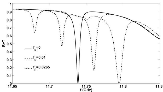
**Figure 12.** Split resonances for the dopant densities  $f_p = 0.01$  (dashed curve) and  $0.0265$  (dash-dotted curve). Here  $\gamma_2 = 0.0008$ . The curve for  $f_p = 0$  (solid curve) is produced for reference. Other parameters are the same as in figure 11.
