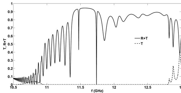
**Figure 11.** CC near the electric plasma frequency of  $M_t$  for normal incidence.  $\epsilon_2 = 3.8$ ,  $\mu_2 = 1$ ,  $d_2 = 21.126$  cm,  $d_1 = 9$  cm and  $d_3 = 15$  cm.
