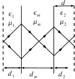
**Figure 6.** Scheme for imaging using a NIM slab (width  $d_m$  and refractive index  $n_m = \sqrt{\epsilon_m \mu_m}$ ). The ambient medium has a refractive index  $n_{1(2)} = \sqrt{\epsilon_{1(2)} \mu_{1(2)}}$  on the object (image) side. The object (‘perfect’ image) plane is at a distance  $d_1$  ( $d_2$ ) from the NIM slab surface.  $d$  is the distance at which the image is observed.
