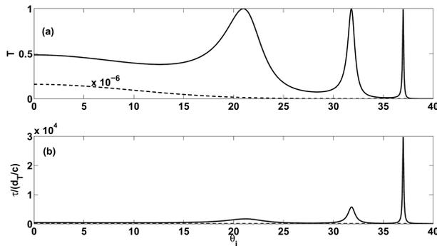
**Figure 5.** (a) Intensity transmission ( $T$ ) and (b) normalized time delay ( $\tau/(d_T/c)$ ) with (solid) and without (dashed) absorption-compensation for guided modes in the NIM guide. The dashed curve in (a) is scaled up by a factor of  $10^6$ . The parameters for the structure are:  $\epsilon_1 = \epsilon_3 = 1$ ,  $d_1 = d_3 = 0.25 \mu\text{m}$  and  $d_2 = 3 \mu\text{m}$ . Other parameters are as in figure 4.
