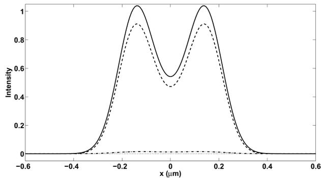
**Figure 9.** Effect of loss on imaging. Images obtained at the ‘perfect’ image plane for  $f = 1$  (dashed curve),  $0.9$  (dash-dotted curve) and  $0$  (dotted curve) compared with the object (solid). Other parameters are same as in figure 7b. Note that for  $f = 0$  the curve is flat and near-zero.
