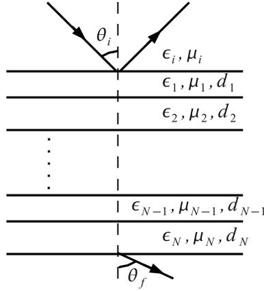
**Figure 1.** Schematic of a layered structure.
