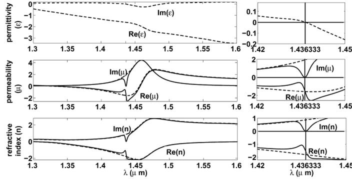
**Figure 3.** Permittivity  $\epsilon$  (top), permeability  $\mu$  (middle) and refractive index  $n$  (bottom) as a function of wavelength ( $\lambda$ ). Their real and imaginary parts are labelled close to the curves. The dashed (solid) curves correspond to the NIM without (with) doping. The right panels are expanded views of the left panels around  $\lambda_0 = 1.436333 \mu\text{m}$  (vertical line). The horizontal line marks the zero value on the vertical axis.
