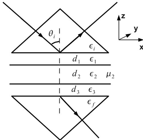
**Figure 2.** Schematic of the layered structure with central NIM layer sandwiched between two spacer layers and high index prisms. All materials except the NIM are assumed to be non-magnetic.
