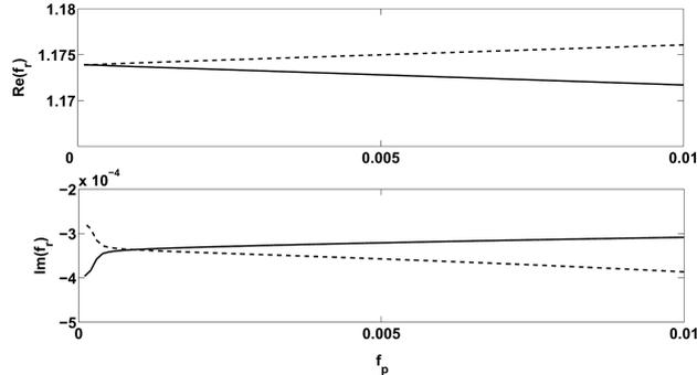
**Figure 13.** The real (top) and imaginary (bottom) parts of the roots of the dispersion relation ( $f_r$ ) of the layered structure as a function of the atomic density at  $\gamma_2 = 0.0008$ . The solid (dashed) curve corresponds to the split resonance at the lower (higher) split frequency.
