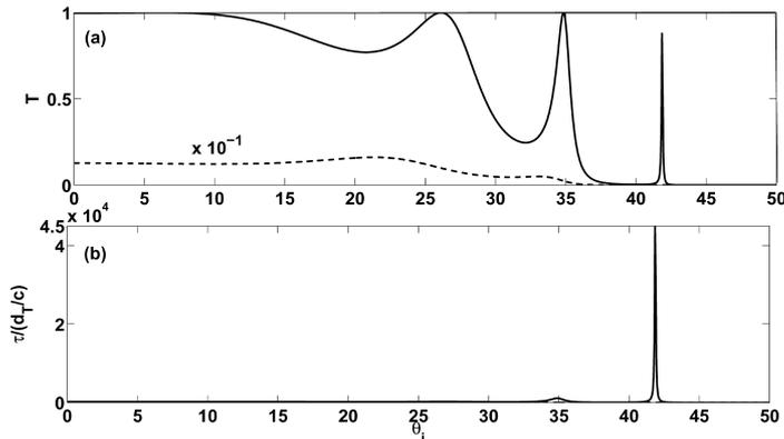
**Figure 4.** (a) Intensity transmission ( $T$ ) and (b) normalized time delay ( $\tau/(d_T/c)$ ) with (solid) and without (dashed) absorption-compensation for plasmon-like modes in the NIM guide. The dashed curve in (a) is scaled up by a factor of 10. The parameters for the structure are  $\epsilon_i = \epsilon_f = 6.145$ ,  $\epsilon_1 = \epsilon_3 = 2.25$ ,  $\mu_i = \mu_f = \mu_1 = \mu_3 = 1$  and  $d_1 = d_3 = 1 \mu\text{m}$ ,  $d_2 = 0.5 \mu\text{m}$ .
