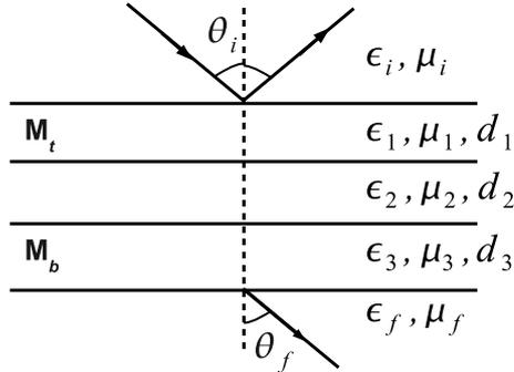
**Figure 10.** Schematic of the layered structure for CC with a dielectric layer of thickness  $d_2$  sandwiched between two MM layers  $M_t$  and  $M_b$ .
