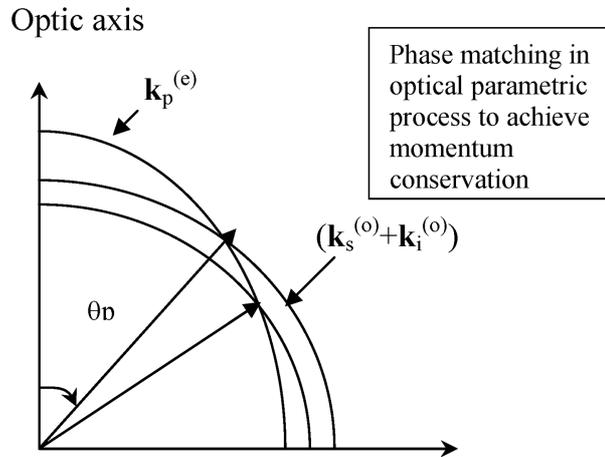
**Figure 1.** Use of birefringence to offset the material dispersion. Rotating the crystal relative to the direction of propagation of the waves leads to tuning of the frequencies of the signal and idler waves.  $\theta_p$  is the phase-matched angle.
