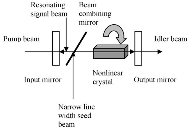
**Figure 2.** Schematic OPO configuration for narrow linewidth radiation by injection seeding technique.
