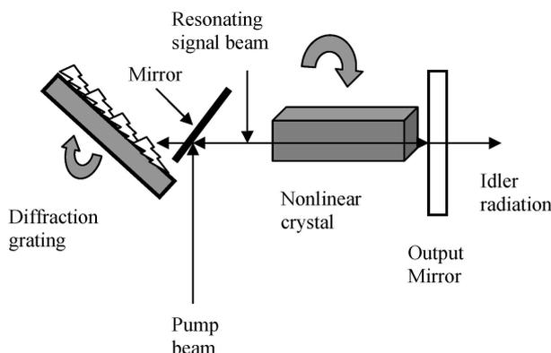
**Figure 3.** Schematic OPO configuration for narrow linewidth radiation incorporating diffraction grating in the cavity.
