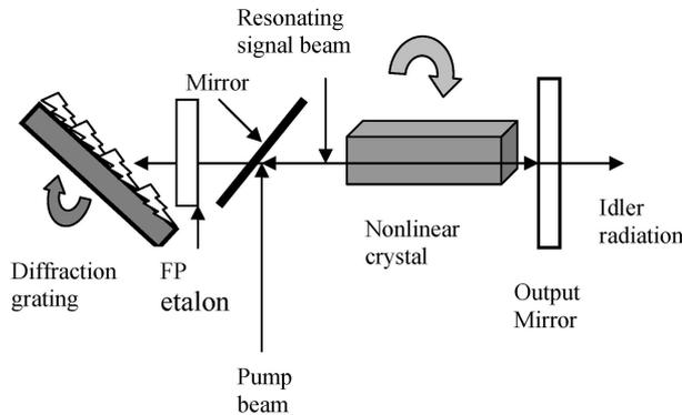
**Figure 4.** Schematic OPO configuration for narrow linewidth radiation incorporating diffraction grating and Fabry–Perot (FP) etalon in the cavity.
