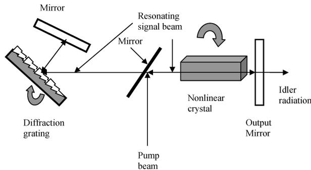
**Figure 5.** Schematic OPO configuration for narrow linewidth radiation incorporating diffraction grating in Littman or grazing angle of incidence configuration.
