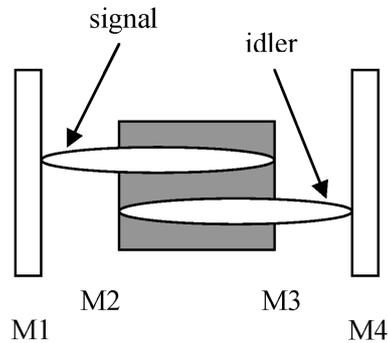
**Figure 6.** Schematic dual or entangled cavity doubly resonant OPO. Mirrors M1 and M3 form the signal cavity while mirrors M2 and M4 form idler cavity.
