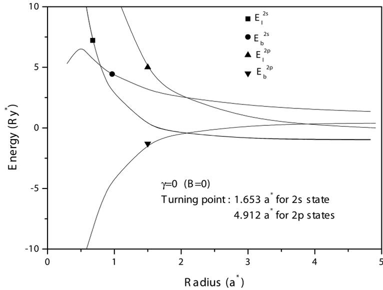
**Figure 1.** The impurity energy ( $E_{IB}$ ) and the binding energy ( $E_b$ ) of the excited states vs. the radius of the finite GaAs/Ga<sub>0.8</sub>Al<sub>0.2</sub>As quantum dot.
