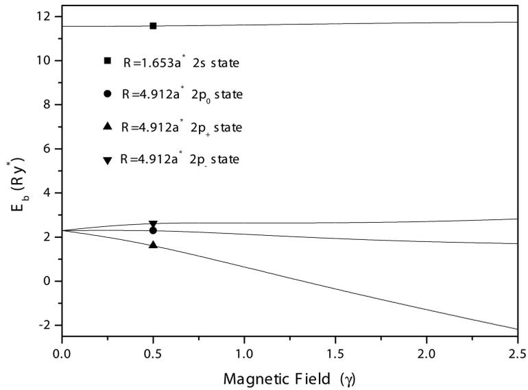
**Figure 4.** The dependence of binding energy ( $E_b$ ) of the excited states vs. magnetic field in finite GaAs/Ga<sub>0.8</sub>Al<sub>0.2</sub>As spherical quantum dots.
