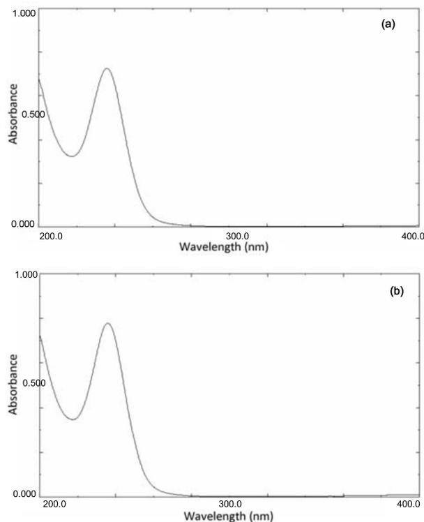
**Figure 4.** (a) Optical absorption spectrum of UTHC crystal and (b) optical absorption spectrum of UTHS crystal.
