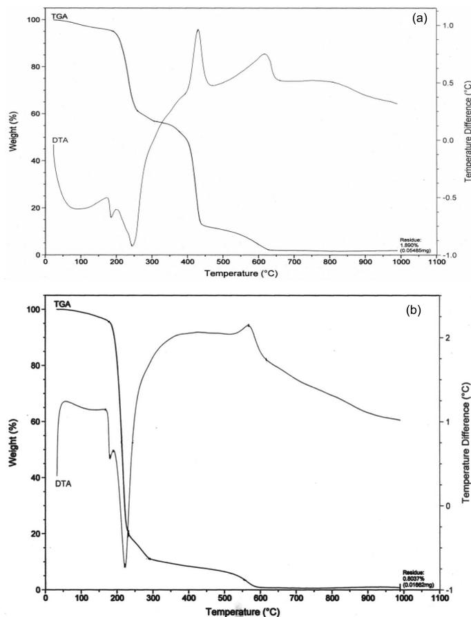
**Figure 5.** (a) Thermogram and differential thermogram of UTHC crystal and (b) thermogram and differential thermogram of UTHS crystal.
