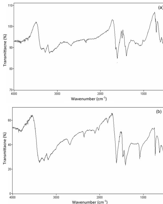
**Figure 6.** (a) FTIR spectrum of UTHC crystal and (b) FTIR spectrum of UTHS crystal.
