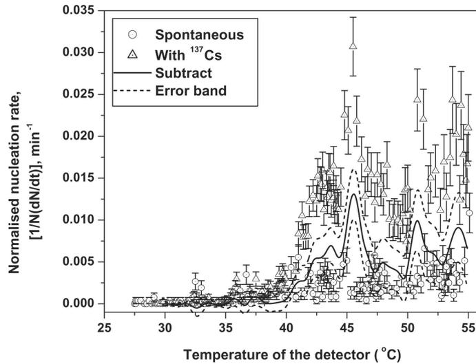
**Figure 3.** The response of R134a detector to  $^{137}\text{Cs}$   $\gamma$ -rays and spontaneous nucleation with varying operating temperatures.
