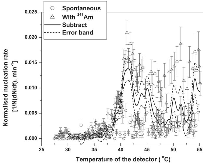
**Figure 2.** The response of R134a detector to  $^{241}\text{Am}$   $\gamma$ -rays and spontaneous nucleation with varying operating temperatures.
