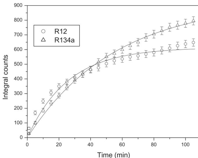
**Figure 1.** The response of superheated emulsion detector of R12 and R134a irradiated with Am–Be neutrons at room temperature. Solid curves are the fitted curves as explained in the text.
