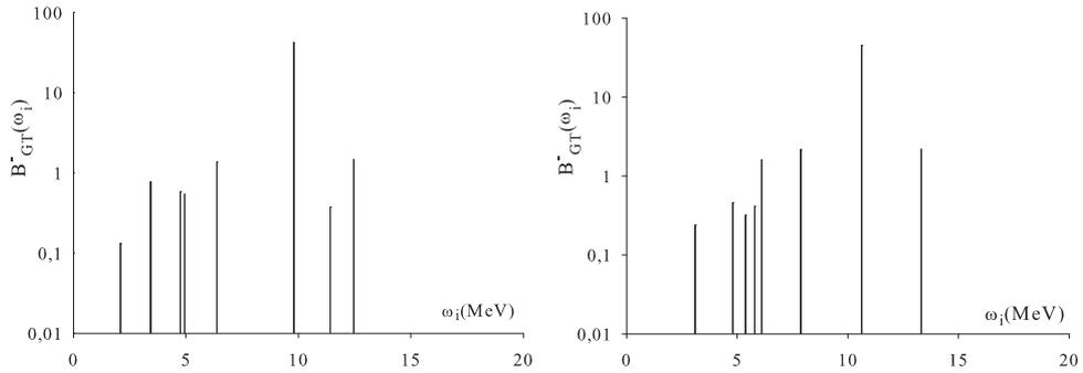
**Figure 2.** GT  $\beta$  transition strength distribution in  $^{116}\text{Sb}$  (left) and  $^{118}\text{Sb}$  (right).
