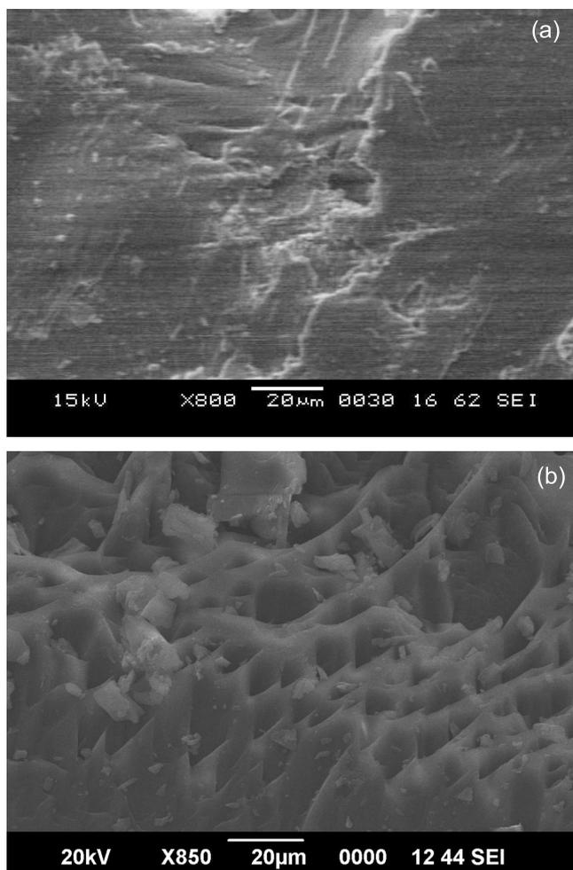
**Figure 4.** SEM micrographs of (a) pristine and (b) electron-irradiated AMIT. Craters are formed on the surface due to irradiation.
