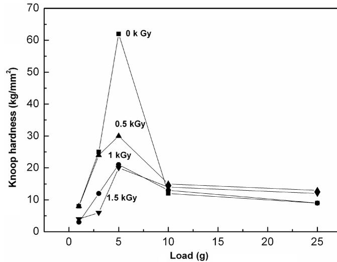
**Figure 2.** Load vs. hardness of AMIT for various electron fluences. Hardness number decreases corresponding to the single peak for a load of 5 g.
