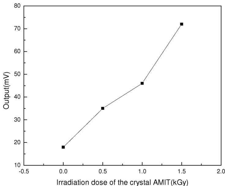
**Figure 3.** SHG response of pristine and irradiated AMIT. SHG increases with absorbed dose.
