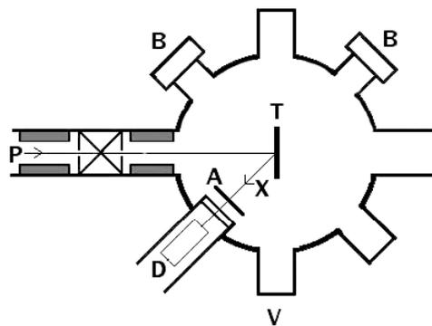
**Figure 1.** Schematic diagram of the experimental set-up for  $\gamma$  attenuation measurements using the PIXE method.
