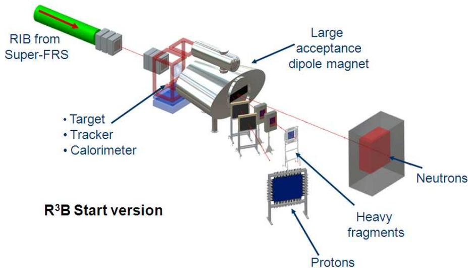
**Figure 3.** Schematic drawing of the R3B experimental set-up comprising  $\gamma$ -ray and target recoil detection, a large-acceptance dipole magnet, a high-resolution magnetic spectrometer, neutron and light-charged particle detectors and a variety of heavy-ion detectors.
