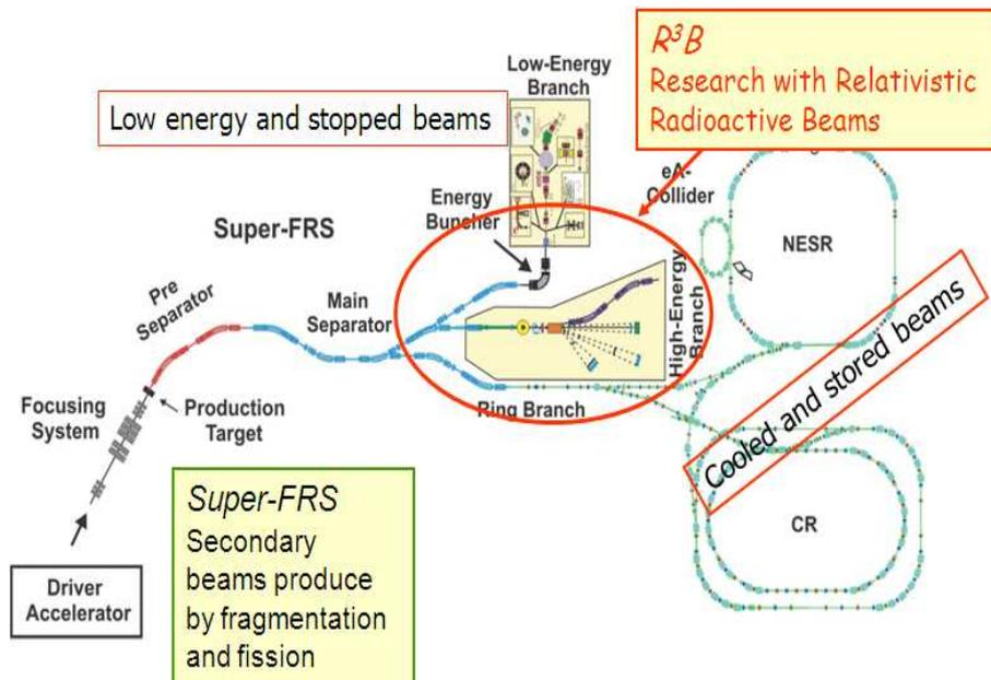
**Figure 2.** Within the FAIR complex, NUSTAR defines a facility where the heart is the super-fragment separator (Super-FRS), which serves three experimental branches: The RING, the LOW- and the HIGH-ENERGY branches.
