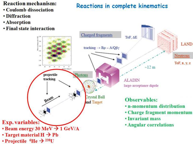
**Figure 4.** Schematic drawing of the LAND experimental set-up, indicating the parameters in a kinematically complete reaction experiment.
