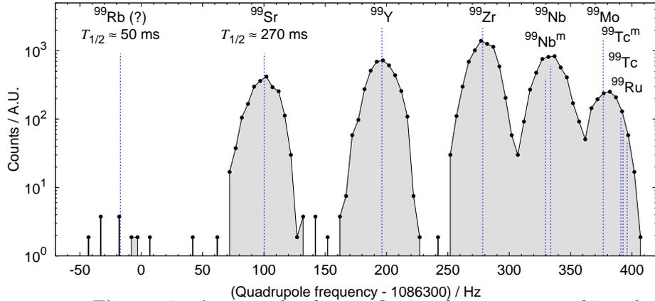
**Figure 2.** An example of a purification frequency scan of ions having  $A/q = 99$  produced in proton induced fission of uranium. Mass resolving power of about  $3 \times 10^4$  is obtained.
