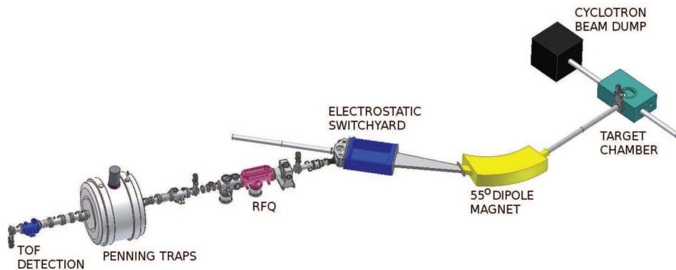
**Figure 1.** Lay-out of the IGISOL and JYFLTRAP installations. The ion guide is housed inside the target chamber (far right). The produced ions are extracted, mass separated with a dipole magnet and steered to the RFQ structure. The cooled and bunched beam from the RFQ is injected to the Penning traps for isobaric/isomeric cleaning and for cyclotron frequency measurement. From the trap, the ions are extracted either to determine their time-of-flight or to perform decay spectroscopy experiments.
