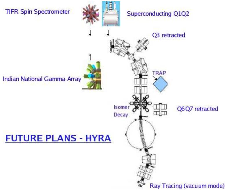
**Figure 8.** Schematic of both stages of HYRA with the various modes of operation and planned add-on facilities.
