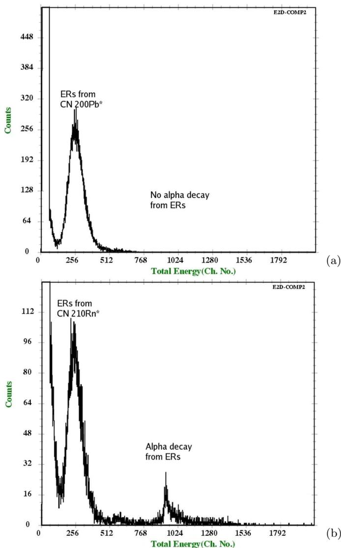
**Figure 4.** (a) Focal plane energy spectrum for  $^{16}\text{O}$  on  $^{184}\text{W}$  with only ERs of low energy seen (no  $\alpha$ -decay is observed in the predominant  $^{194,195}\text{Pb}$  residues). (b) Focal plane energy spectrum for  $^{16}\text{O}$  on  $^{194}\text{Pt}$  with ERs of low energy and  $\alpha$ -decay of higher energy observed in the predominant  $^{204,205}\text{Rn}$  residues.
