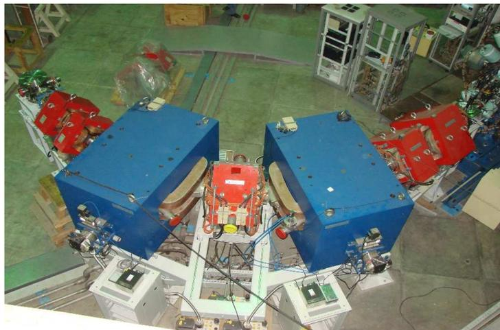
**Figure 1.** First stage of HYRA spectrometer used in gas-filled mode (particles enter from right).
