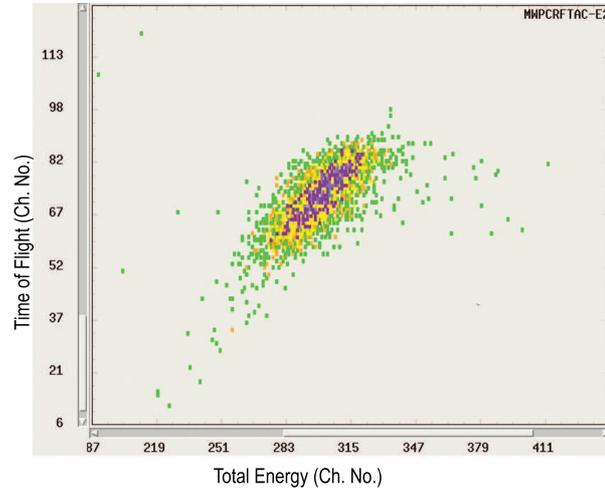
**Figure 6.** Forward moving elastic recoils from  $^{48}\text{Ti}$  on  $^{\text{nat}}\text{Pb}$  at an energy below barrier selected using gas-filled mode of HYRA as seen in total energy vs. time-of-flight spectrum.
