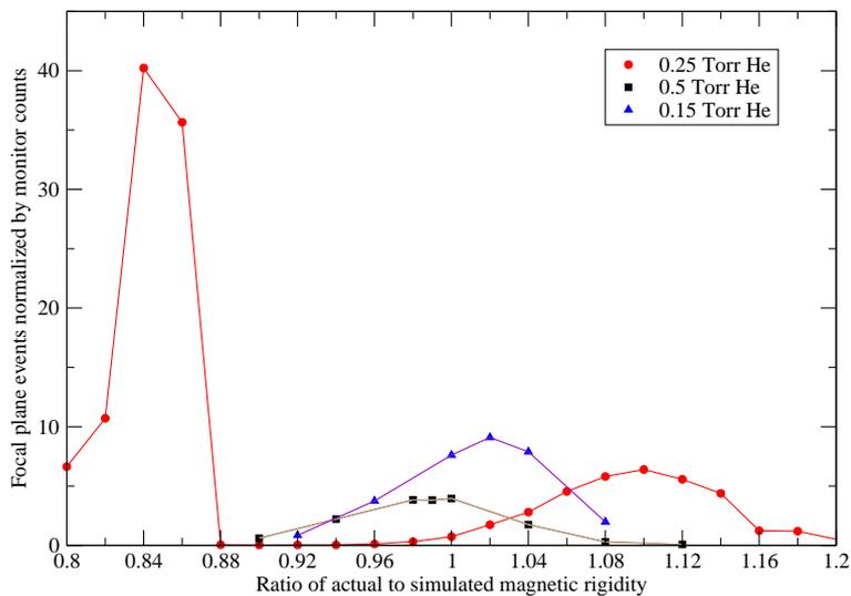
**Figure 3.** Normalized ER counts at the focal plane as a function of the ratio of actual to simulated magnetic rigidity for 0.5 Torr, 0.25 Torr and 0.15 Torr helium gas pressure settings in HYRA. Lines joining the points are to guide the eye.
