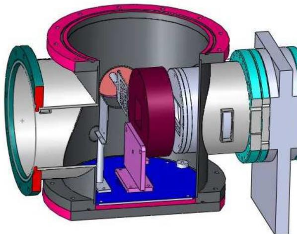
**Figure 2.** Schematic of focal plane detector system used in gas-filled mode of HYRA showing gate valve, window foil to separate helium and isobutane sections, MWPC detector, retractable shutter and silicon stop detector; residues enter from the right.
