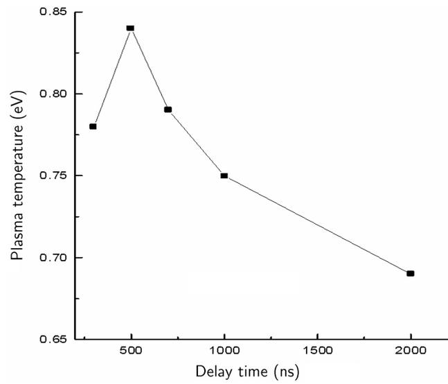
**Figure 5.** Variation of plasma temperature with delay time.
