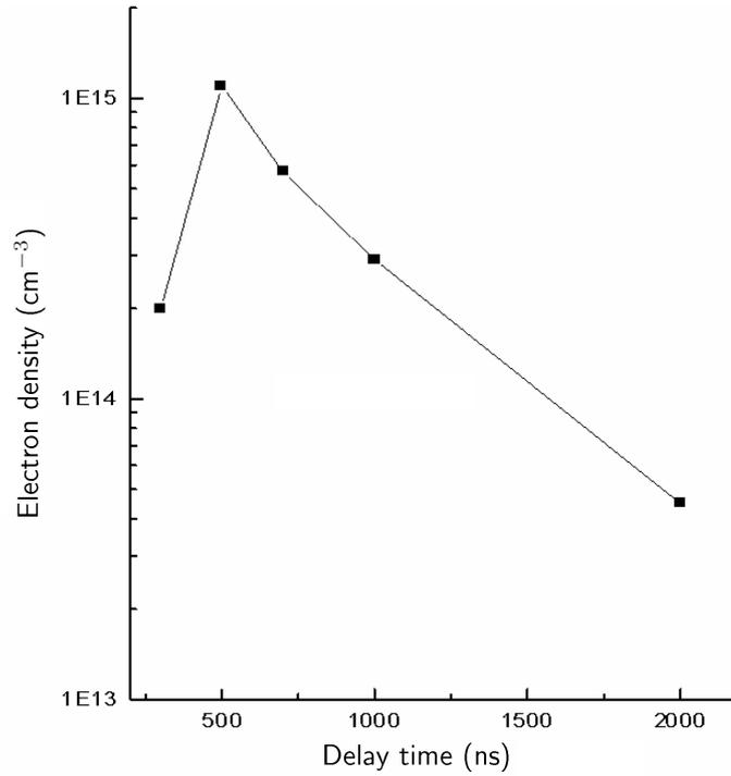
**Figure 6.** Variation of electron density with delay time.
