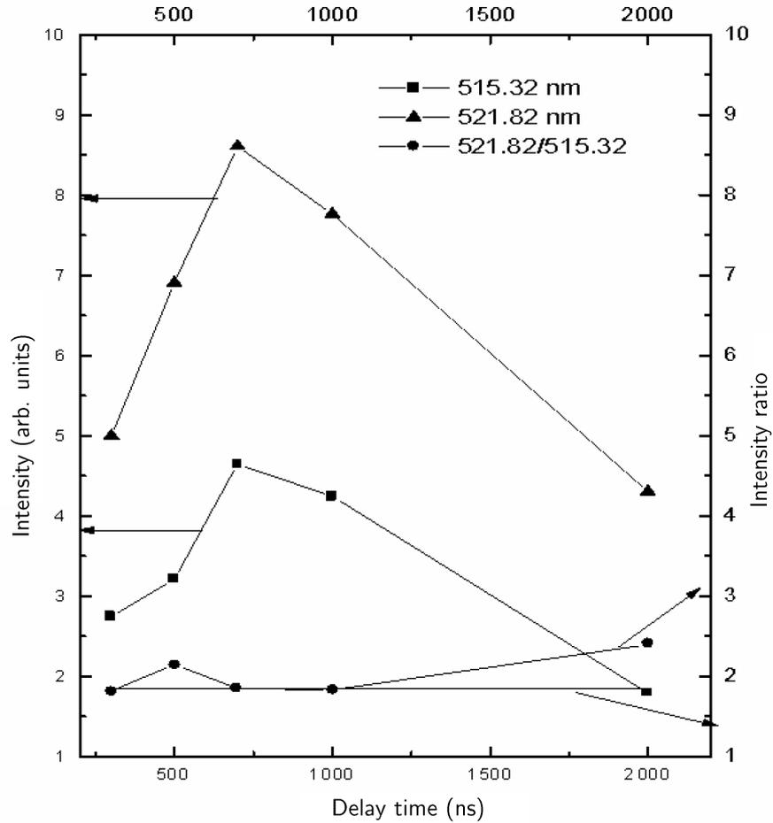
**Figure 7.** Temporal evolution of intensities of two Cu I lines 515.32 and 521.82 nm and their intensity ratio. The straight line indicates the theoretical intensity ratio = 1.85 for this couple of lines, which is the condition of an optically thin and LTE plasma. The time window for the thin and LTE plasma is 700–1000 ns.
