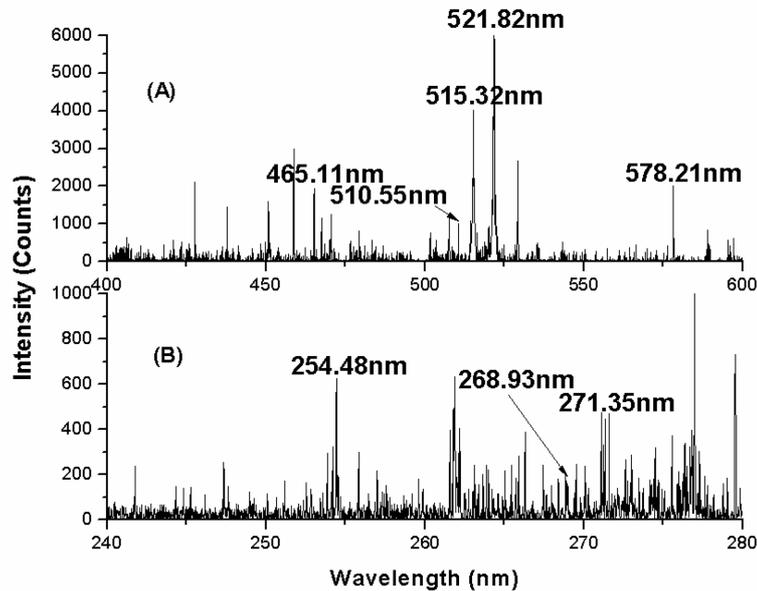
**Figure 3.** LIBS spectra of copper recorded using ICCD-based echelle spectrograph with a gate delay time of 700 ns at a laser irradiance of  $4.5 \times 10^8 \text{ W/cm}^2$ , showing (A) Cu I atomic lines and (B) Cu II ionic lines used for the characterization of the laser-induced Cu plasma.
