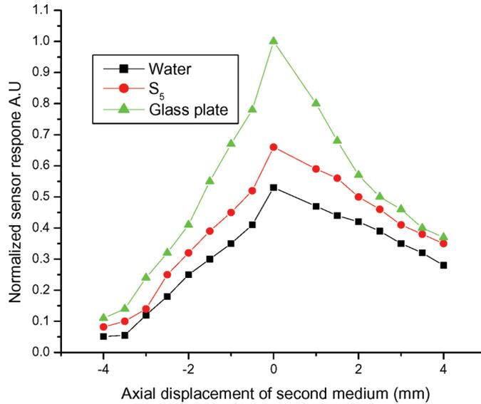
**Figure 3.** Representation of the sensor response with axial displacement for three different mediums.
