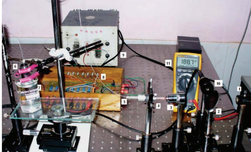
**Figure 2.** Photograph of the experimental set-up for a non-intrusive refractometer. 1 – diode laser, 2 – beam splitter, 3 – objective, 4 – fibre holder, 5 – optical fibre, 6 – objective, 7 – liquid sample, 8 – amplifier, 9 – power supply, 10 – photodiode, 11 – digital multimeter.
