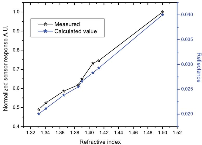
**Figure 4.** Theoretical and measured reflectances of light signal for different refractive mediums.
