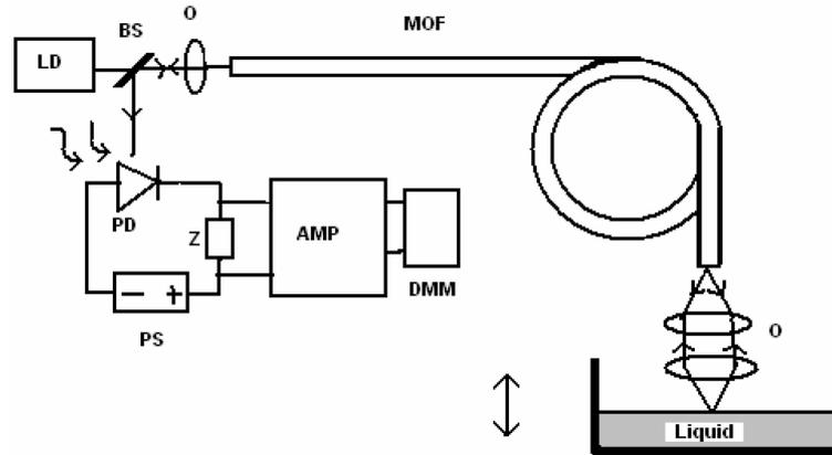
**Figure 1.** Schematic configuration of the experimental set-up. LD – Laser diode, BS – beam splitter, O – objective, MOF – multimode optical fibre, PD – photodiode, PS – power supply, Z – impedance, AMP – amplifier, DMM – digital multimeter.
