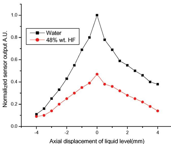
Figure 5. Normalized sensor response for water and 48% wt. HF solution.
