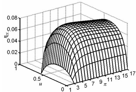
**Figure 10.** Comprehensive relationships among exergetic efficiency, distribution of heat conductance and pressure ratio.
