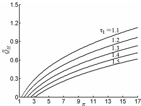
**Figure 3.** Effect of heat reservoir temperature ratio on the dimensionless heating load vs. pressure ratio.
