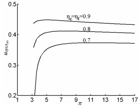
**Figure 14.** Effect of efficiencies of the compressor and expander on the optimum distribution of heat conductance vs. pressure ratio.
