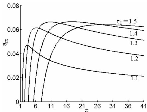
**Figure 2.** Effect of heat reservoir temperature ratio on the exergetic efficiency vs. pressure ratio.
