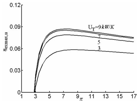
**Figure 17.** Effect of total heat exchanger inventory on the maximum exergetic efficiency vs. pressure ratio.
