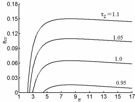
**Figure 7.** Effect of the ratio of hot-side heat reservoir temperature to ambient temperature on the exergetic efficiency vs. pressure ratio.
