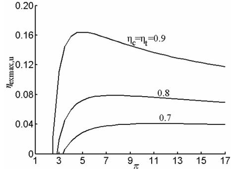
**Figure 18.** Effect of efficiencies of the compressor and expander on the maximum exergetic efficiency vs. pressure ratio.
