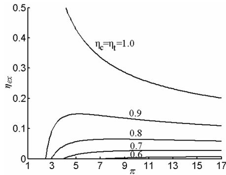
**Figure 6.** Effect of efficiencies of the compressor and expander on the exergetic efficiency vs. pressure ratio.
