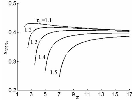
**Figure 12.** Effect of heat reservoir temperature ratio on the optimum distribution of heat conductance vs. pressure ratio.
