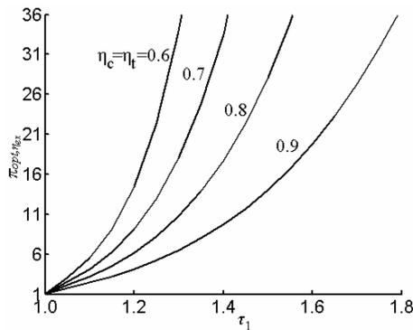
**Figure 9.** Effect of efficiencies of the compressor and expander on the optimum pressure ratio vs. heat reservoir temperature ratio.
