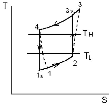
**Figure 1.** Temperature–entropy diagram of an irreversible heat pump working on reversed Brayton cycle with constant temperature heat reservoirs.
