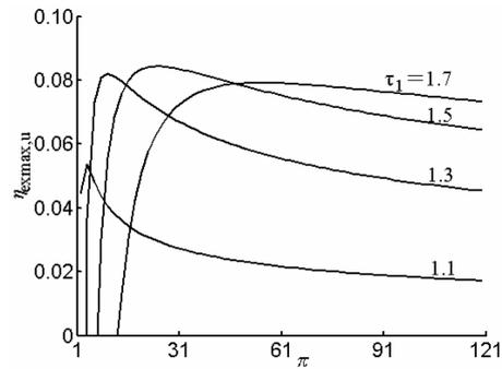
**Figure 16.** Effect of heat reservoir temperature ratio on the maximum exergetic efficiency vs. pressure ratio.
