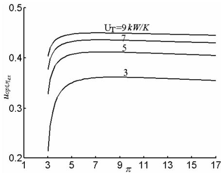
**Figure 13.** Effect of total heat exchanger inventory on the optimum distribution of heat conductance vs. pressure ratio.
