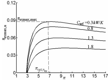
**Figure 15.** Effect of thermal capacity rate of the working fluid on the maximum exergetic efficiency vs. pressure ratio.
