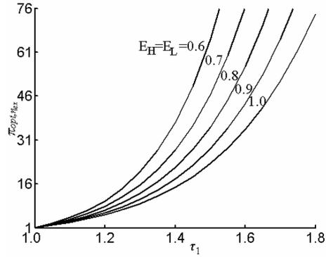
**Figure 8.** Effect of effectivenesses of the heat exchangers on the optimum pressure ratio vs. heat reservoir temperature ratio.
