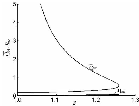
**Figure 4.** Exergetic efficiency and the dimensionless heating load vs. the COP.
