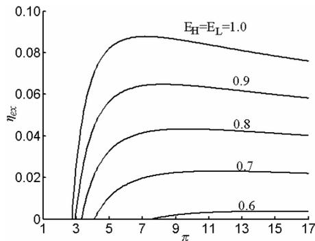
**Figure 5.** Effect of effectivenesses of the heat exchangers on the exergetic efficiency vs. pressure ratio.
