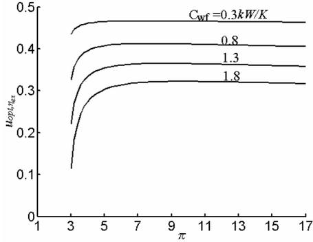
**Figure 11.** Effect of thermal capacity rate of the working fluid on the optimum distribution of heat conductance vs. pressure ratio.
