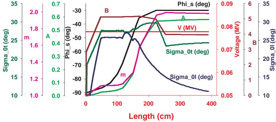
Figure 1. RFQ parameters along the length for design D1.
