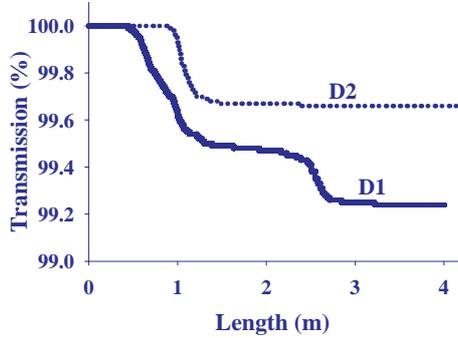
**Figure 3.** Transmission along the RFQ length for D1 and D2.
