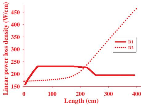
**Figure 7.** Linear power loss density (W/cm) along the length of RFQ.
