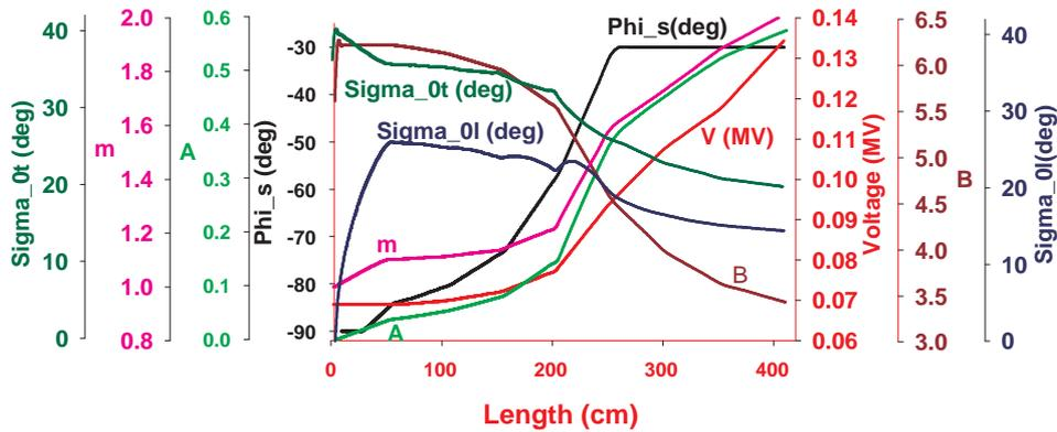
**Figure 2.** RFQ parameters along the length for design D2.
