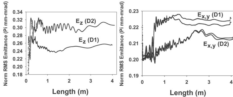
**Figure 6.** Variation of normalized r.m.s. emittance for D1 and D2 along the RFQ length.
