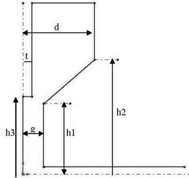
**Figure 9.** Schematic of the vane undercut.
