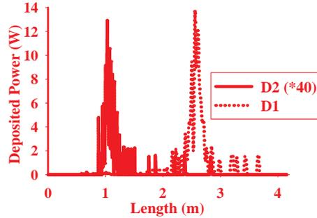
**Figure 4.** Power deposited due to beam loss along the RFQ length for D1 and D2.
