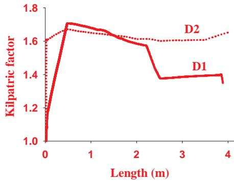
**Figure 5.** Kilpatrick factor for design D1 and D2 along the RFQ length.
