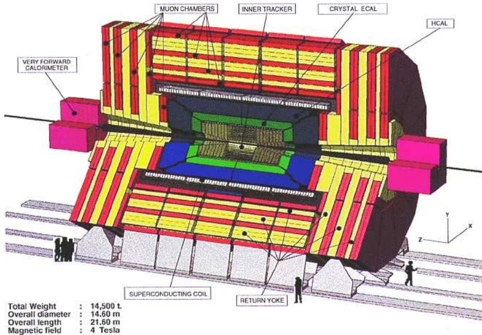
Figure 1. Three-dimensional overview of the CMS detector.
