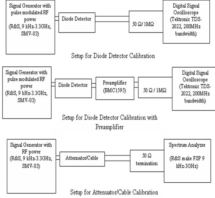
Figure 5. Calibration set-up of HPM diagnostic components.
