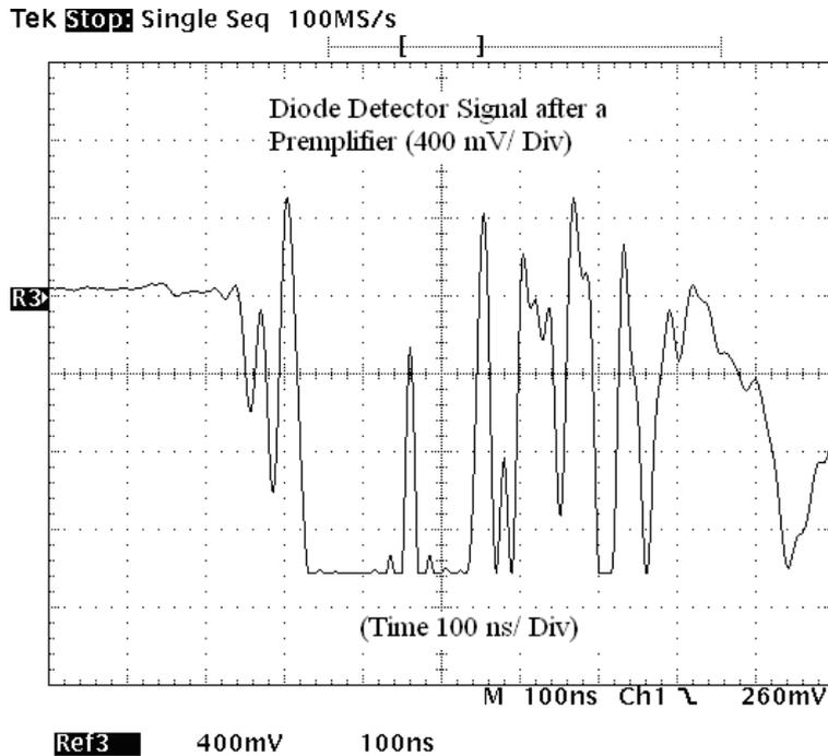
**Figure 9.** Diode detector signal after a preamplifier is used when the BNC cable is kept inside a metal conduit.
