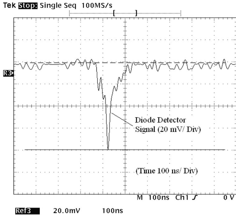
**Figure 10.** HPM signal from the diode detector when measured with an RF cable.
