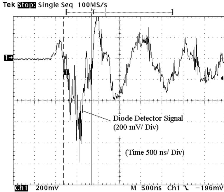
Figure 7. HPM signal after detection when carried to the scope by a BNC cable.
