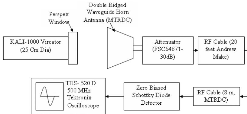
**Figure 11.** HPM diagnostics set-up by which HPM signal has been measured successfully in the presence of significant electrical high frequency noise.
