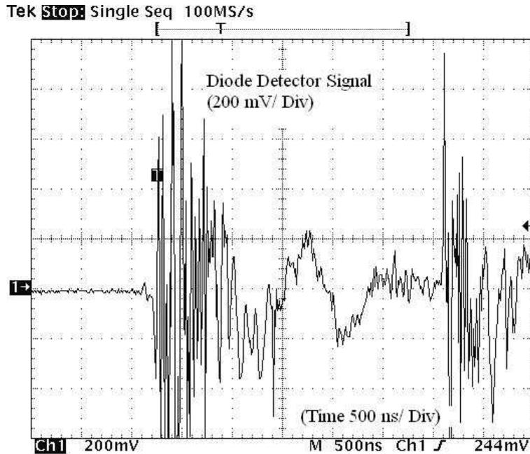
**Figure 8.** Diode detector signal when the BNC cable is kept inside a metal conduit.
