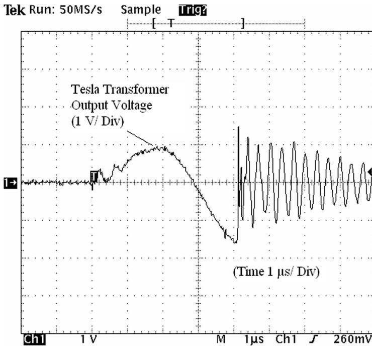
Figure 3. Tesla transformer output signal.
