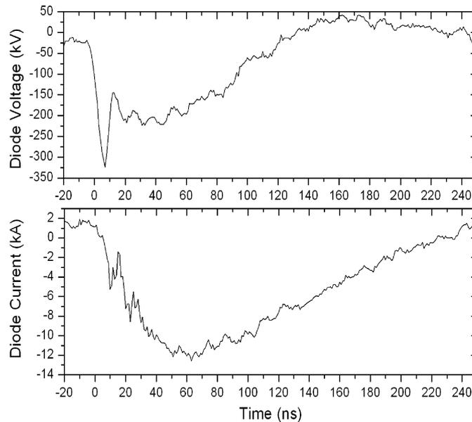
**Figure 4.** Electron beam diode voltage and current waveform for 6 mm A–K gap with 70 mm diameter graphite cathode.
