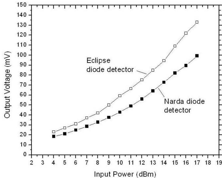
**Figure 6.** Calibration curve of the Eclipse and Narda make diode detectors using standard modulated RF source at 2 GHz.
