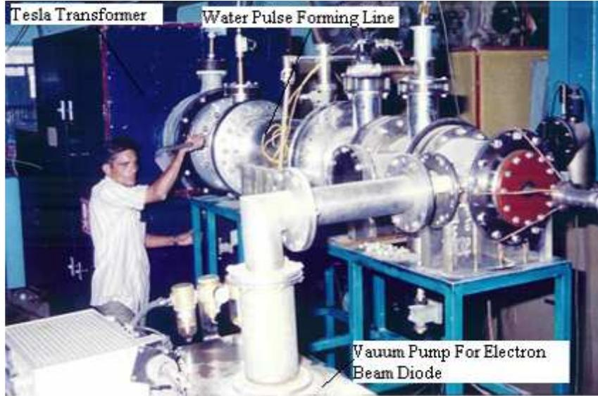
**Figure 1.** A photograph of the KALI-1000 pulse power system.
