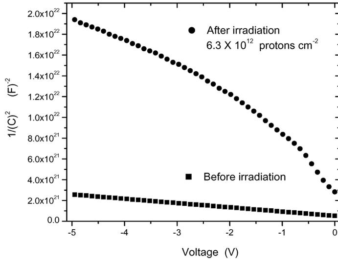
**Figure 3.** Capacitance–voltage characteristics of the base–collector junction of the transistor before and after proton irradiation.
