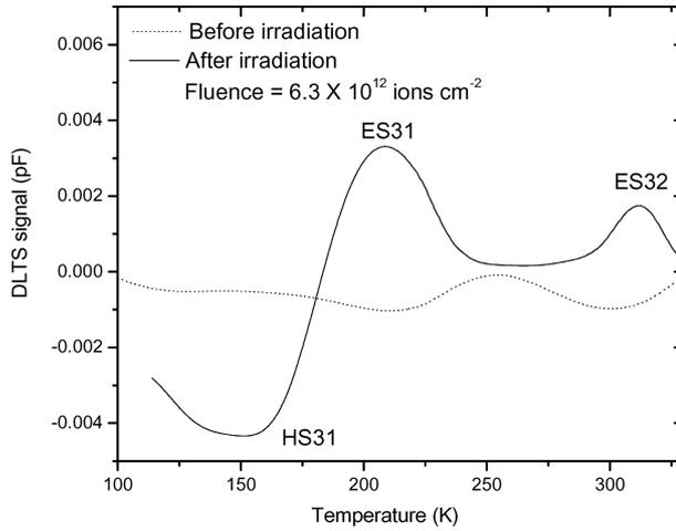
**Figure 5.** DLTS spectrum of 24 MeV proton-irradiated transistor. Rate window is fixed at  $51.7 \text{ s}^{-1}$ .
