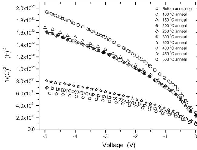
**Figure 4.** Capacitance–voltage characteristics of the base–collector junction of the proton-irradiated transistor after isochronal (30 min) annealing at different temperatures.
