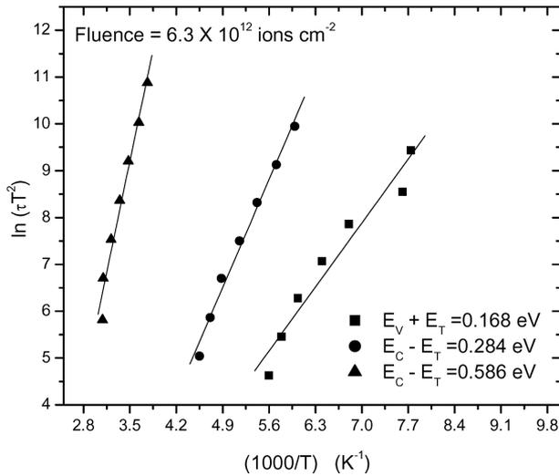
**Figure 6.** Arrhenius plots for the 24 MeV proton-irradiated transistor.
