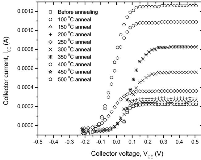
**Figure 2.** Collector characteristics of the proton-irradiated transistor after isochronal (30 min) annealing at different temperatures (at constant  $I_B = 50 \mu\text{A}$ ).
