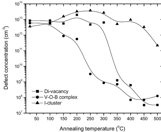
**Figure 7.** Variation of defect concentration as a function of isochronal (30 min) annealing temperature in the proton-irradiated transistor.
