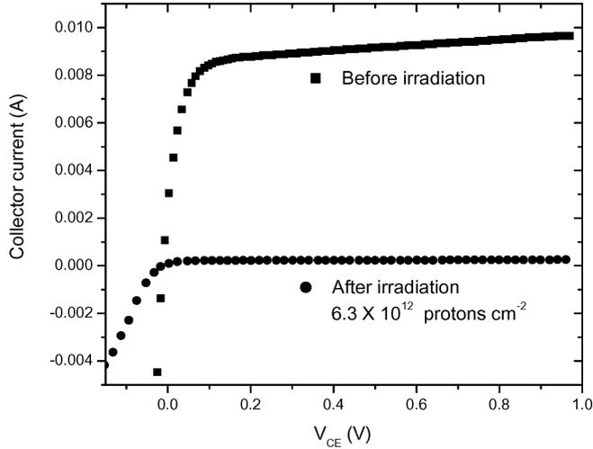
**Figure 1.** Collector characteristics of the transistor before and after the proton irradiation (at constant  $I_B = 50 \mu\text{A}$ ).
