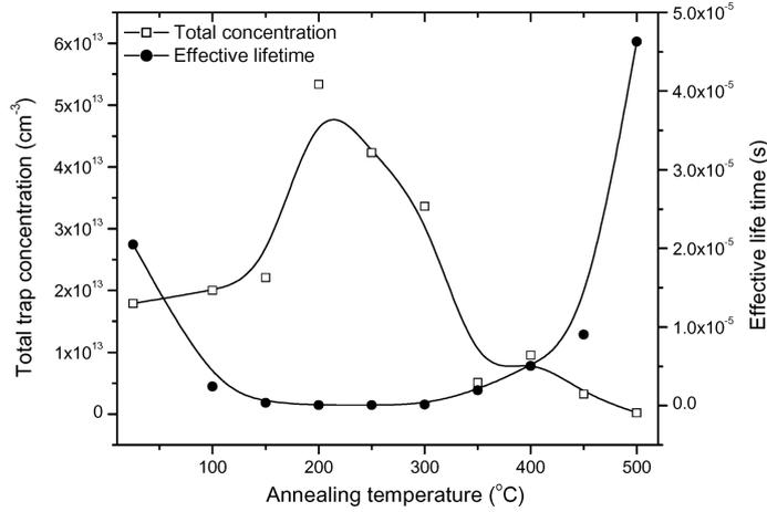
**Figure 8.** Variation of total trap concentration and effective lifetime as a function of isochronal (30 min) annealing temperature in the proton-irradiated transistor.
