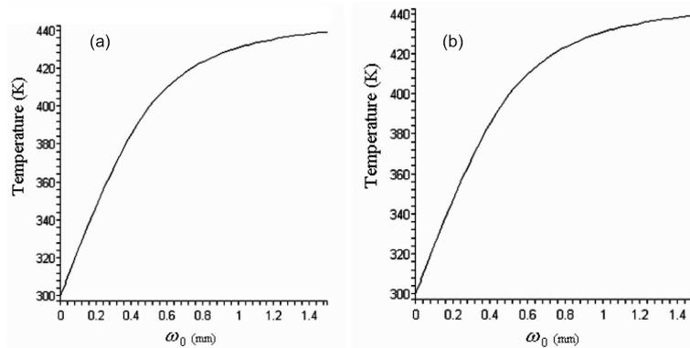
**Figure 6.** Maximum temperature in the crystal vs.  $\omega_0$ . (a) In equal double pumping with  $P_1 = P_r = 5$  W, (b)  $P_1 = P_r = 100$  W.
