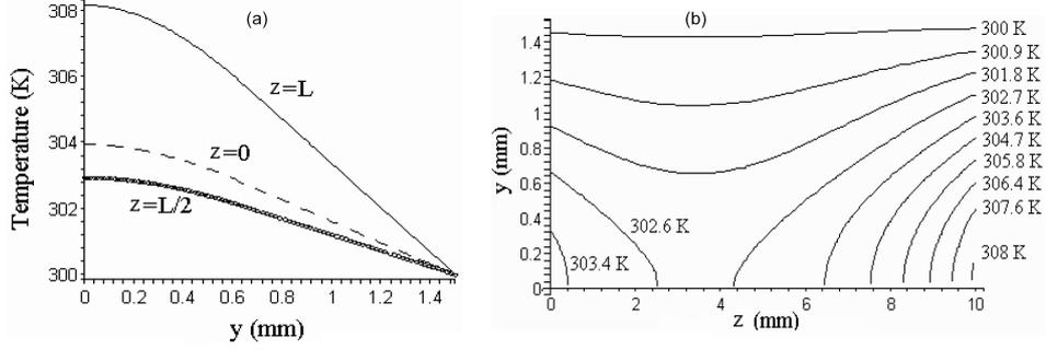
**Figure 2.** Temperature distributions in double-end-pumped cubic crystal. The left and right input power is 3 W and 7 W respectively. (a) Temperature along  $y$ -direction at  $z = 0, L/2, L$ . (b) Contour graph.
