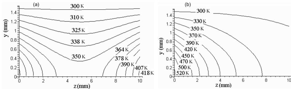
**Figure 5.** Contour plot of temperature distribution in (a) double equal pumping with  $P_1 = P_r = 100$  W and (b) single pumping with  $P = 200$  W.
