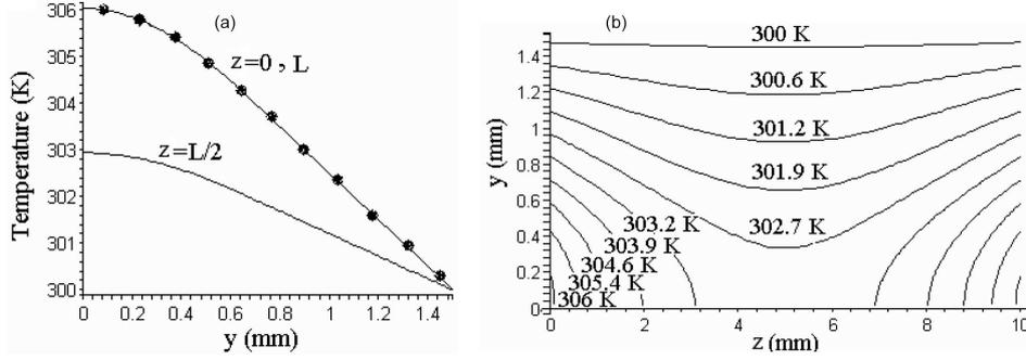
**Figure 3.** Temperature distributions in double-end-pumped crystal. The left and right input power is 5 W. (a) Temperature along  $y$ -direction at  $z = 0, L/2, L$ . (b) Contour graph.
