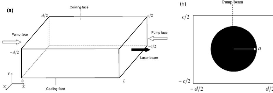
**Figure 1.** Schematic diagram of the double-end-pumped cubic crystal: (a) The pump beam of the crystal is along the  $z$ -direction and heat is removed from four sides of the surfaces. (b) Pump dimension on the  $x$ - $y$  plane.
