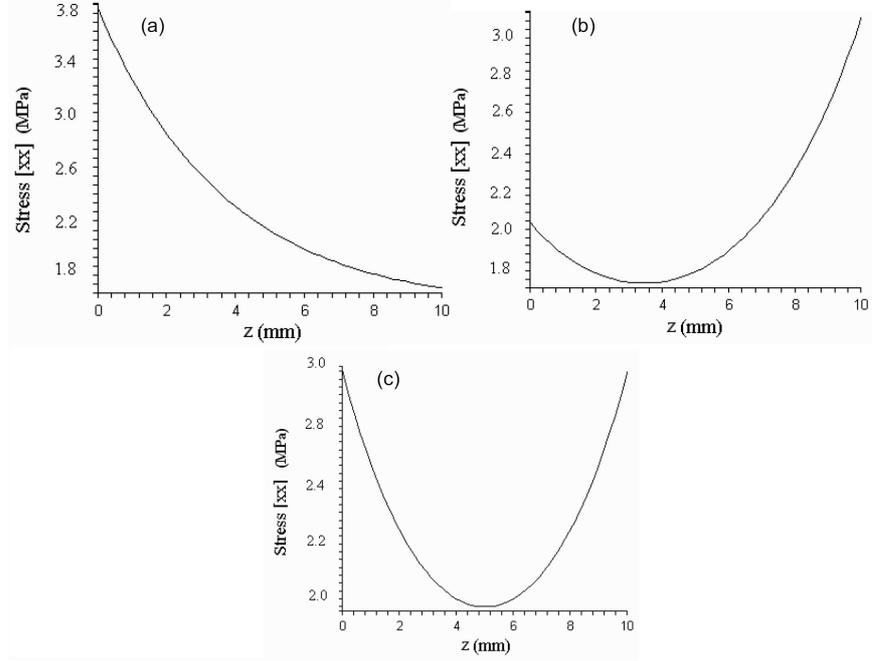
**Figure 7.**  $\sigma_{xx}$  component of stress vs.  $z$  in  $y = 0$ . (a) Single pump with  $P_1 = 10$  W, (b) double pump with  $P_1 = 3$  W and  $P_r = 7$  W and (c) double pump with  $P_1 = P_r = 5$  W.
