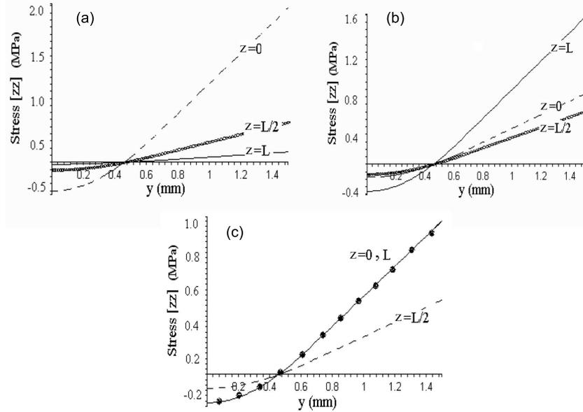
**Figure 8.**  $\sigma_{zz}$  component of stress vs.  $y$  in  $x = 0$ . (a) Single pump with  $P_1 = 10$  W, (b) double pump with  $P_1 = 3$  W and  $P_r = 7$  W and (c) double pump with  $P_1 = P_r = 5$  W.
