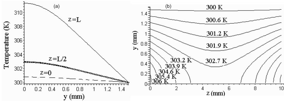
**Figure 4.** Temperature distributions in single-end-pumped crystal: (a) Temperature along  $y$ -direction at  $z = 0, L/2, L$ . (b) Contour graph.
