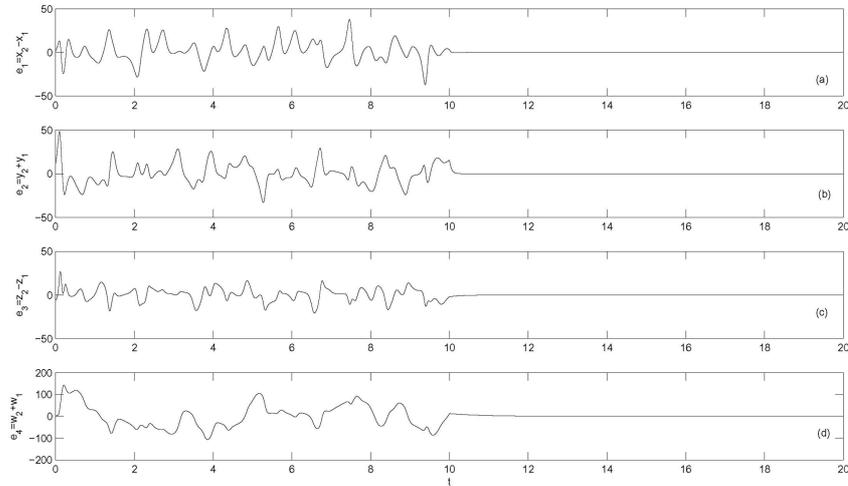
**Figure 3.** Time response of error states  $e_1, e_2, e_3$  and  $e_4$  with active control law activated after 10 s. (a) Error signal  $e_1 = x_2 - x_1$ , (b) error signal  $e_2 = y_2 + y_1$ , (c) error signal  $e_3 = z_2 - z_1$  and (d) error signal  $e_4 = w_2 + w_1$ .
