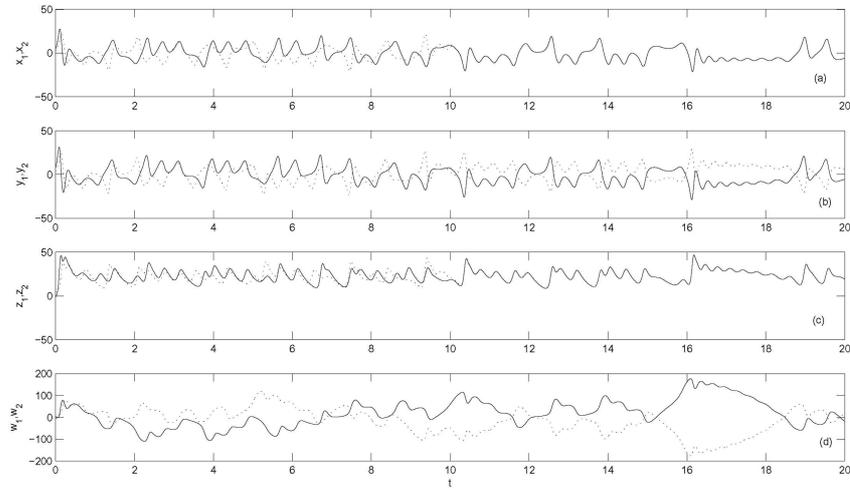
**Figure 2.** Time response of states for the drive system  $(x_1, y_1, z_1, w_1)$  and response system  $(x_2, y_2, z_2, w_2)$  with active control law activated after 10 s. (a) Signals  $x_1$  and  $x_2$ , (b) signals  $y_1$  and  $y_2$ , (c) signals  $z_1$  and  $z_2$  and (d) signals  $w_1$  and  $w_2$ .
