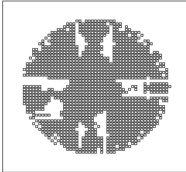
**Figure 10.** Simulated fingering pattern for a plane plate under the same conditions as for figures 5 and 6. The pattern developed in 5 time-steps shows much slower growth of fingers than for the grooved plates.
