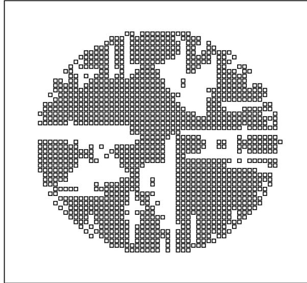
**Figure 2.** A viscous fingering pattern generated by simulation of the lifting process or constant force, with viscosity parameter 0.014.
