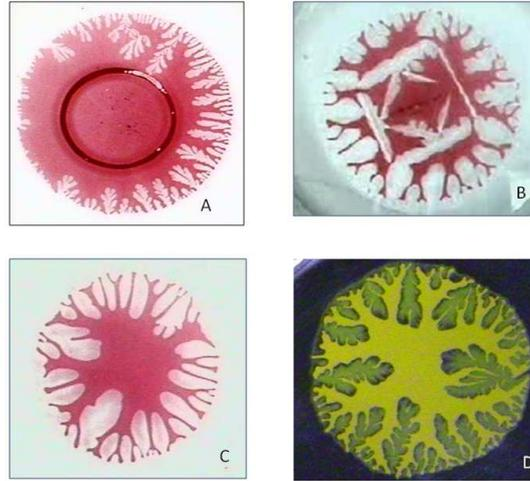
**Figure 1.** Experimentally obtained fingers for (A) circular grooved plate, (B) square grooved plate, (C) plane plate with a Newtonian fluid and (D) plane plate with a non-Newtonian fluid.
