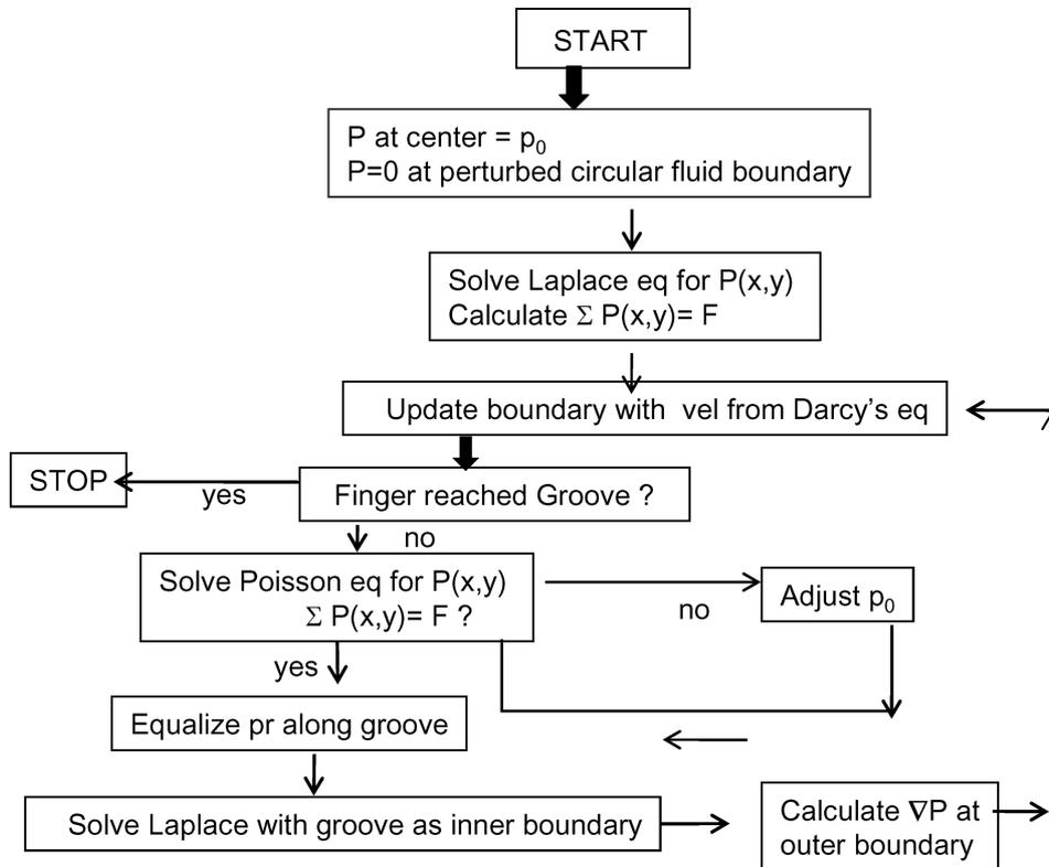
**Figure 4.** Flow chart illustrating the sequence of steps followed for the simulation of the grooved patterns.
