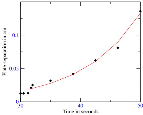
**Figure 8.** Experimental plate separation as a function of time is represented by the symbols, and the line is the exponential fit.
