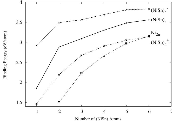
**Figure 3.** Binding energy per atom (eV) for neutral, ionic  $(\text{NiSn})_n$  ( $n = 1-6$ ) and  $\text{Ni}_{2n}$  [16] clusters vs. number of  $(\text{NiSn})$  atoms in the cluster.
