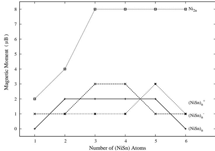
**Figure 7.** Total magnetic moment (in  $\mu\text{B}$ ) for the neutral, ionic  $(\text{NiSn})_n$  ( $n = 1-6$ ) and the  $\text{Ni}_{2n}$  [16] structures as a function of the number of (NiSn) atoms in the cluster.
