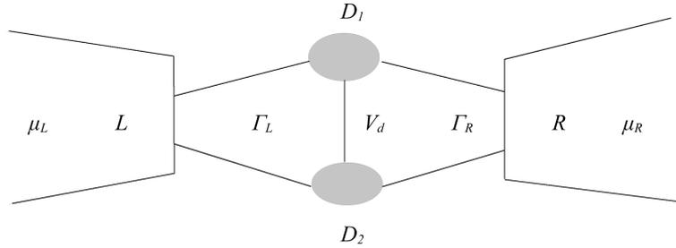
**Figure 1.** Schematic display of a parallel coupled quantum dot system. The two dots  $D_1$  and  $D_2$ , are coupled to the left (L) and right leads (R) by tunnel barriers with coupling strengths  $\Gamma_L$  and  $\Gamma_R$  respectively. Here  $V_d$  is the inter-dot coupling strength and  $\mu_{L(R)}$ , the chemical potential of the left (right) lead.
