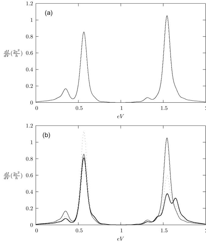
**Figure 5.** (a) The differential conductance as a function of  $eV$  of parallel CQD at  $U = 1$ ,  $U' = 0.1U$ ,  $\Gamma = 0.08U$ ,  $\varepsilon = 0.4U$ ,  $kT = 0.025U$  and  $V_d = 0$ . (b) The differential conductance vs. bias voltage of parallel CQD at  $U = 1$ ,  $U' = 0.1U$ ,  $\Gamma = 0.08U$  and  $\varepsilon = 0.4U$ . Thin line stands for  $V_d = 0$ , thick dotted line stands for  $V_d = 0.06U$  and thick line stands for  $V_d = 0.1U$ .
