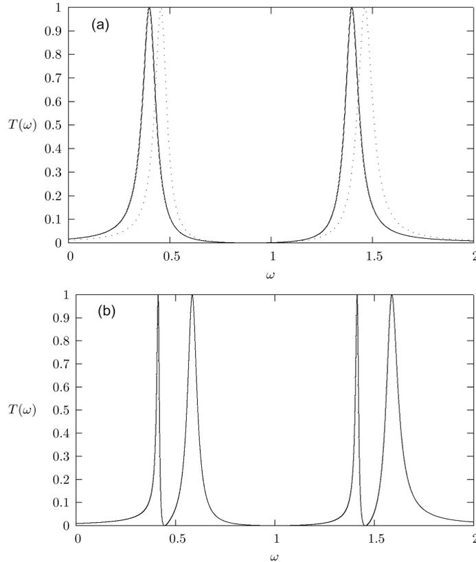
**Figure 2.** (a) The  $T(\omega)$  vs.  $\omega$  graph of parallel CQD at  $U = 1$ ,  $\Gamma = 0.08U$  and  $\varepsilon = 0.4U$ . Solid line denotes  $V_d = 0$  and dotted line denotes  $V_d = 0.12U$ . (b) The  $T(\omega)$  vs.  $\omega$  graph of parallel CQD at  $U = 1$ ,  $\Gamma = 0.08U$  and  $\varepsilon = 0.4U$ ,  $V_d = 0.1U$  and  $U' = 0.1U$ .
