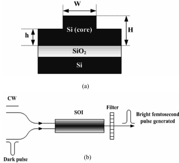
**Figure 1.** Schematic diagrams of (a) cross-section of SOI ridge waveguide and (b) the operation principle for the generation of ultrafast pulse.
