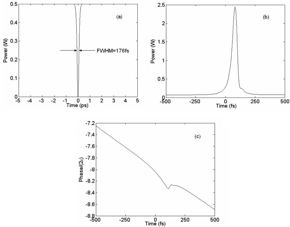
**Figure 2.** (a) The input ultrafast dark pulse, (b) the ultrafast pulse generated at the end of 5-mm long waveguide and (c) the phase profile of the generated pulse.
