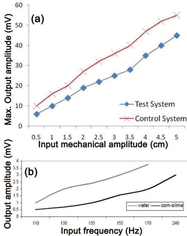
**Figure 2.** Maximum output amplitude of transmitted vibrations against input amplitude for (a) test and control systems for oscillator system and (b) water and corn-flour slime systems. It is obvious from the figure that both the test system of oscillators as well as the corn-flour system exhibited a lower output amplitude.
