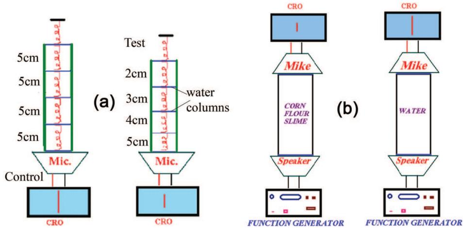
**Figure 1.** Schematic diagram of the experiments to detect (a) directional energy damping in an oscillator system with a frequency gradient and (b) shock-absorbing properties in corn-flour slime.
