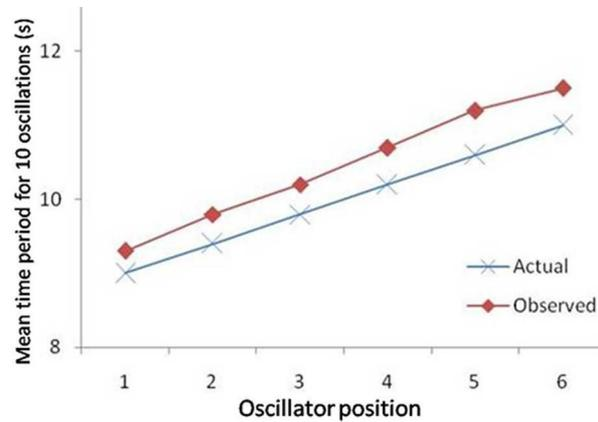
**Figure 3.** Plot of variation of time period of successive oscillators in the test system of oscillators as a function of oscillator position. The figure shows that observed frequencies vary in tune with the theoretical values suggesting that the oscillators retained their natural frequency.
