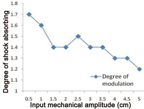
**Figure 4.** The variation of degree of modulation as the input mechanical amplitude of the ‘test’ system is increased. The degree of modulation was calculated as the ratio of output amplitudes in the test and control systems of oscillators. It can be seen that the degree of shock absorbing decreases as the amplitude increases.
