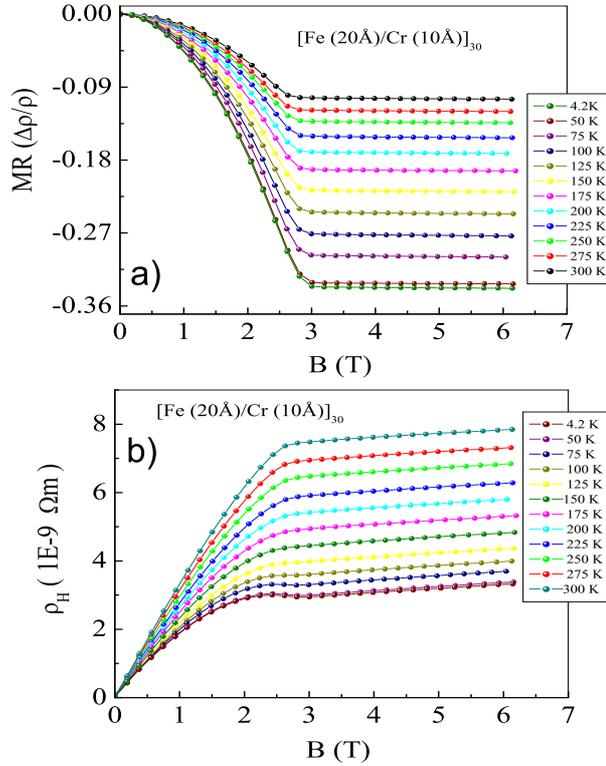
**Figure 3.** Plots of (a) magnetoresistance (MR) vs. field  $B(T)$  and (b) Hall resistivity ( $\rho_H$ ) vs. field  $B(T)$ , measured at various temperatures on a Fe/Cr GMR multilayer sample. The solid lines are just guides to the eye.
