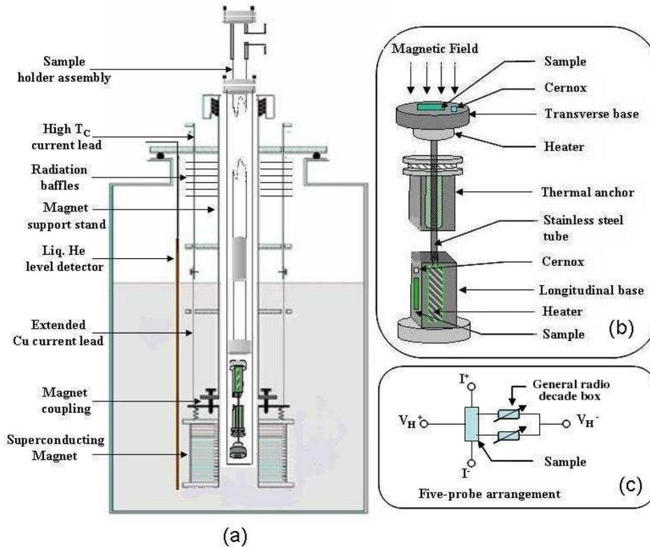
**Figure 1.** Schematic diagram of (a) the magnetotransport set-up consisting of a 6.5 T superconducting magnet and a variable temperature sample holder assembly, (b) a detailed design of the sample holder for electrical measurements in longitudinal and transverse orientations of the samples with respect to the magnetic field and (c) a five-probe arrangement for Hall effect measurements.
