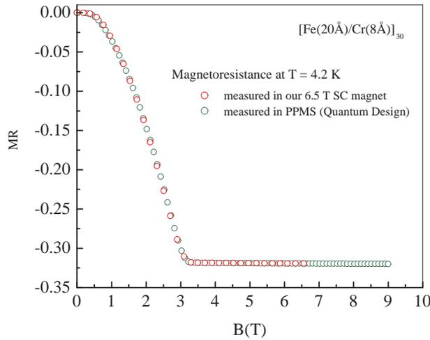
**Figure 2.** Magnetoresistance vs.  $B(T)$  of a Fe/Cr GMR multilayer sample measured using our 6.5 T magnet system and a commercial 14 T quantum design PPMS for comparison. The excellent match between the two plots shows the degree of accuracy of the field calibration of our superconducting magnet.
