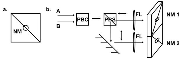
**Figure 1.** The optical switch and the structure of the optical router. Attention: The reflector will affect the position of polarization light beams, but the polarization light beams can still cause the nonlinear effect. NM – the nonlinear medium, FL – the focussing lens.
