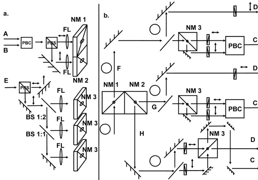
**Figure 4.** The whole computing scheme. (a) The scheme of the adapted controlling terminal. (b) The scheme of the adapted output terminal.
