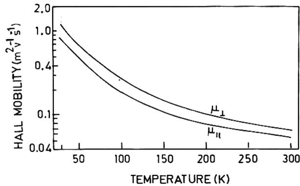
**Figure 1.** Temperature variation of Hall mobility for  $L_z = 10.5$  nm,  $N_{2D} = 4.8 \times 10^{15} \text{ m}^{-2}$ ,  $N_i = 8.6 \times 10^{22} \text{ m}^{-3}$ , and  $B = 0.002$  T.  $\mu_{\parallel}$  and  $\mu_{\perp}$  represent mobilities with piezoelectric parallel mode and perpendicular mode scatterings, respectively, and including all other scattering mechanisms.
