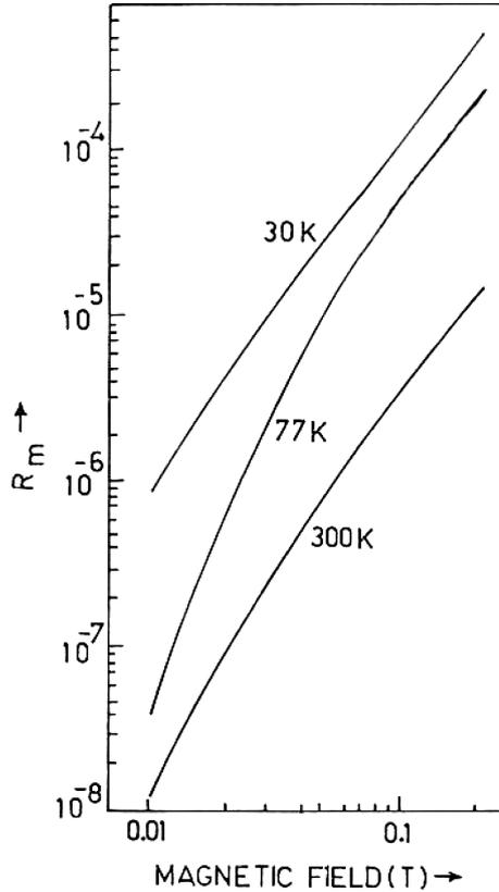
**Figure 3.** Magnetoresistance coefficient ( $R_m$ ) vs. magnetic field for 30, 77, and 300 K. The other parameter values are the same as in figure 1.
