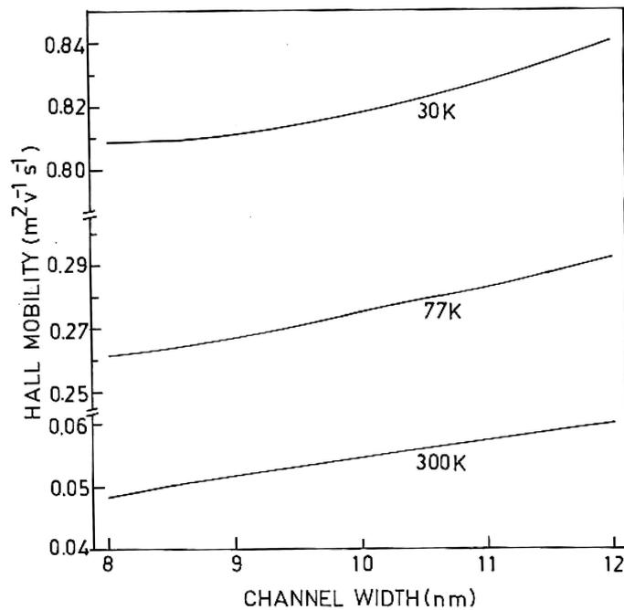
**Figure 2.** Hall mobility vs. channel width for 30, 77, and 300 K. The other parameter values are the same as in figure 1.
