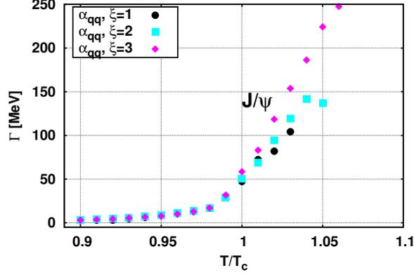
**Figure 4.** Thermal width of  $J/\psi$  obtained from the second-order Stark effect and QCD sum rule constraint.
