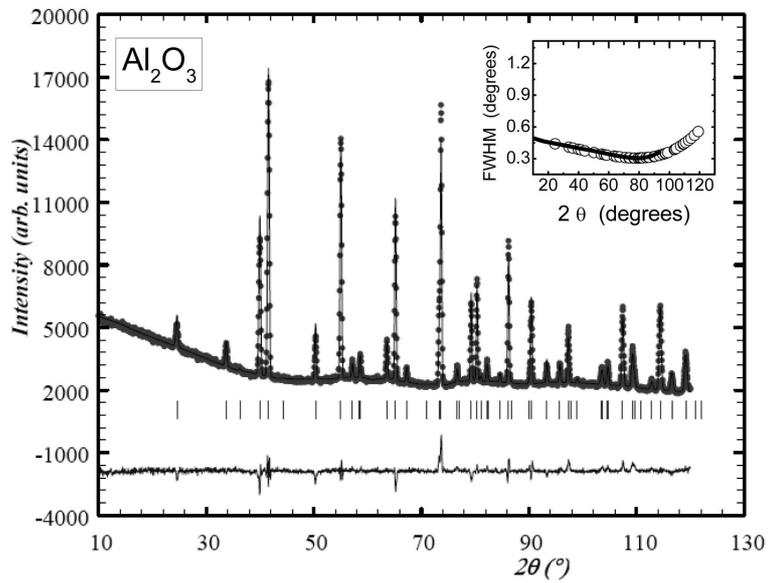
**Figure 3.** Rietveld refinement of sintered  $\text{Al}_2\text{O}_3$  rod. Inset shows the  $2\theta$  dependence of FWHM obtained from Rietveld analysis (open circles) and Monte Carlo simulation (solid line) (ref. [6]).
