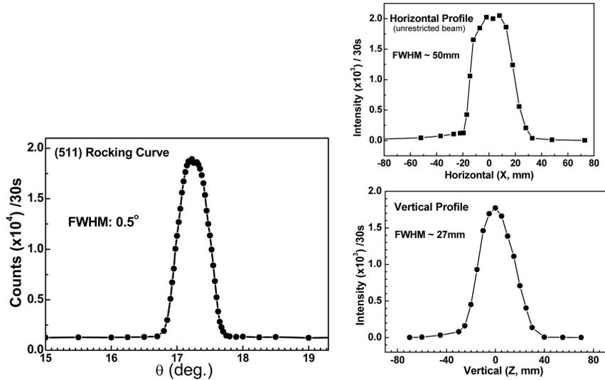
**Figure 2.** Rocking curve of bent perfect Si monochromator at a take-off angle of  $90^\circ$  and  $\lambda = 1.48 \text{ \AA}$ . Figures on right show the horizontal and vertical beam profiles measured at sample position.
