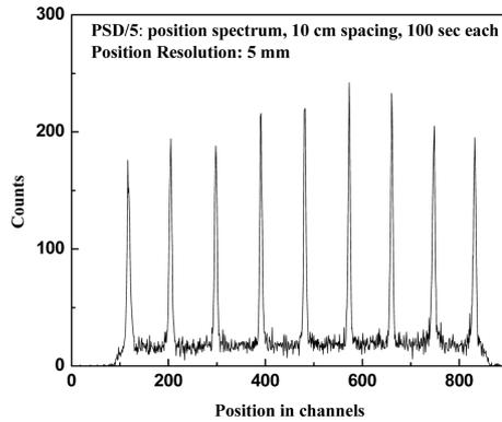
**Figure 3.** Position spectrum with 1.5 mm collimated beam with a shift of 10 cm.
