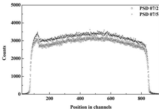
**Figure 2.** Flood pattern showing the uniformity of efficiency for PSDs with Pu–Be source exposed parallel to the detector length. Data for only 2 of the 5 PSDs are shown for the sake of clarity.
