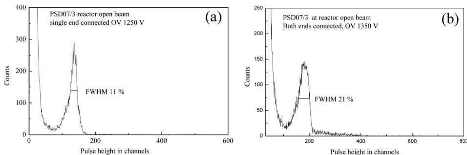
**Figure 1.** Pulse height spectra of a PSD with (a) single and (b) both ends connected.
