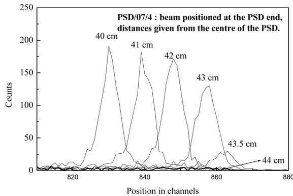
**Figure 6.** Position spectrum showing end effects on peak width and efficiency at the extreme end of the PSD.
