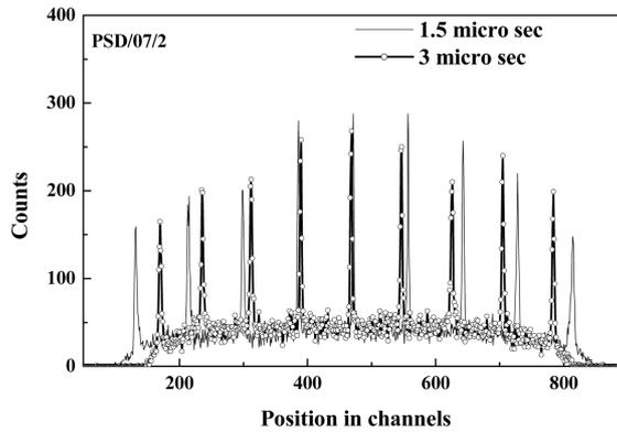
**Figure 4.** Position spectra showing the effect of amplifier shaping time on the dynamic range.
