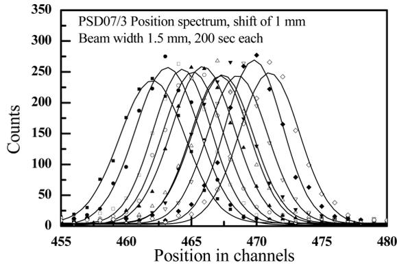
**Figure 5.** Position spectra of a PSD with collimated neutron beam and shift of 1 mm along the length.
