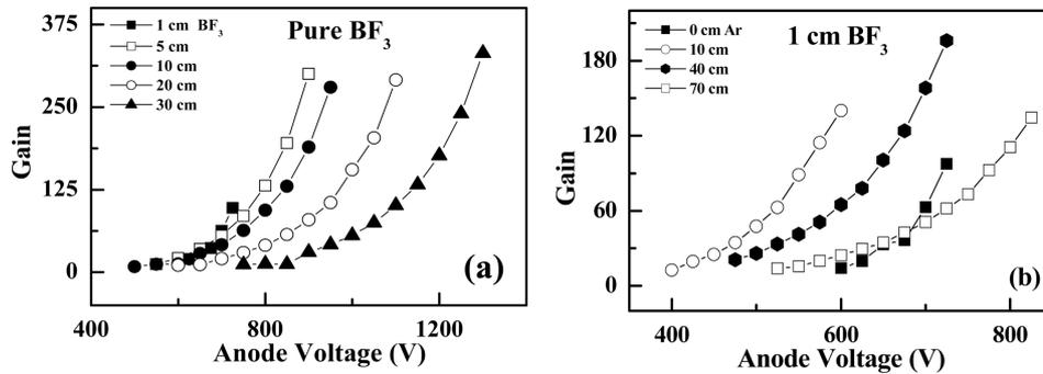
Figure 2. Variation of gas gain with applied voltage for various pressure fillings of BF<sub>3</sub> + Ar.
