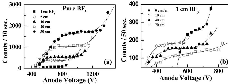
**Figure 3.** Plateau characteristics curves for counters filled with various pressures of BF<sub>3</sub> and Ar.
