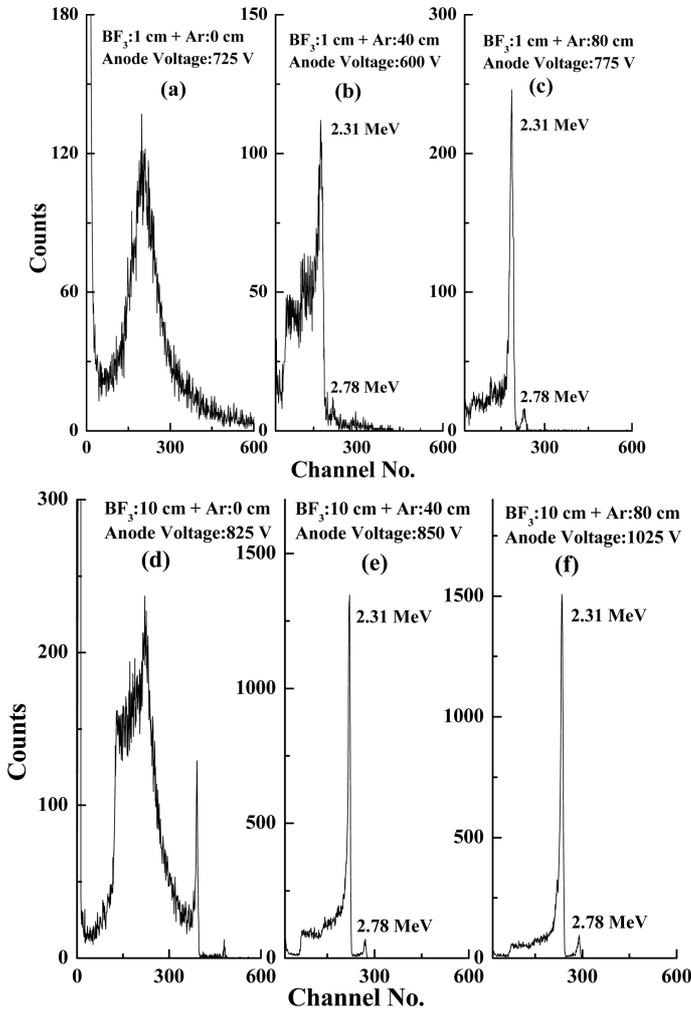
**Figure 1.** Pulse height distribution curves of counters with various BF<sub>3</sub> and Ar pressures.
