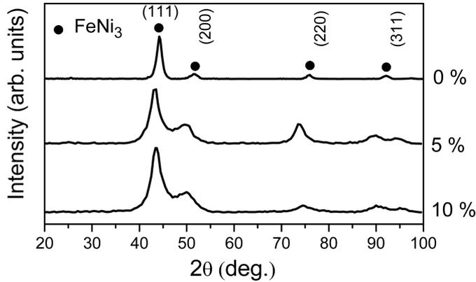
**Figure 1.** X-ray diffraction pattern of NiFe samples prepared with different amounts of reactive nitrogen during sputtering.
