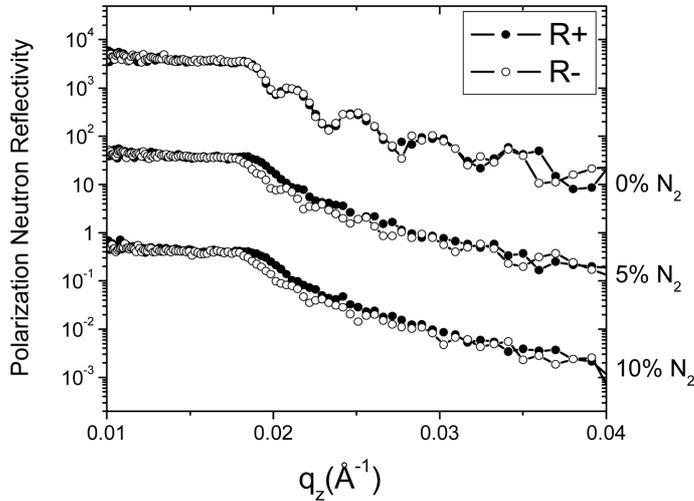
**Figure 3.** Polarized neutron reflectivity measurements of NiFe samples prepared with different amounts of reactive nitrogen during sputtering. Note that the intensity at the  $y$ -axis has been multiplied by a factor of 100 for clarity.
