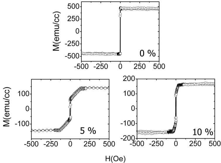
**Figure 2.** Magnetization measurements of NiFe samples prepared with different amounts of reactive nitrogen during sputtering.
