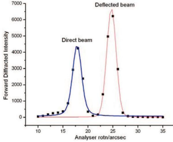
**Figure 3.** Voigt function fits (curves) to the direct and deflected beam scans (points).
