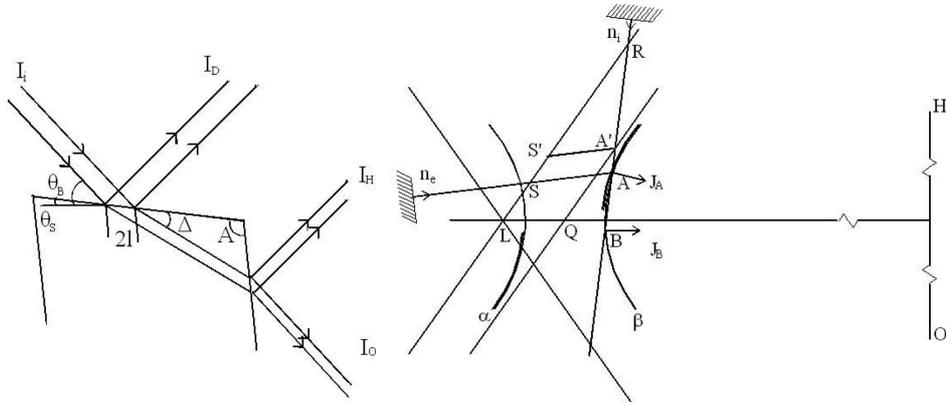
**Figure 1.** Bragg diffraction of a neutron beam from a thick single crystal in real and reciprocal spaces.
