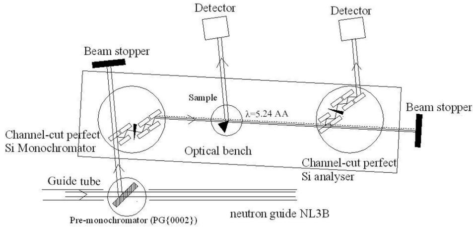
**Figure 2.** Experimental lay-out for the determination of  $\delta_{cr}$  and  $I_o$ .
