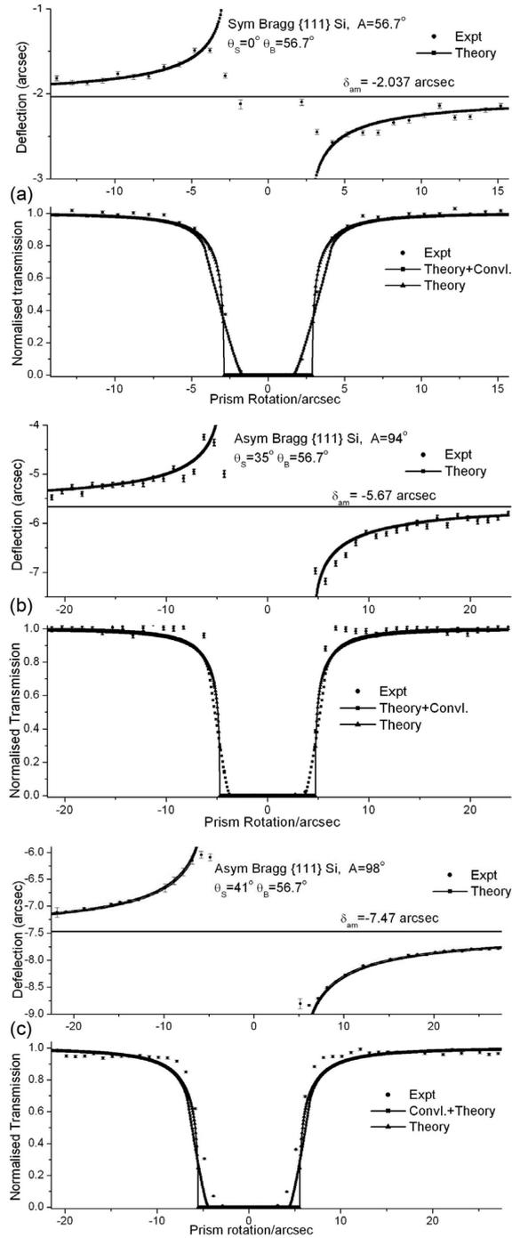
**Figure 4.** Deflection and transmitted intensity fraction of neutrons forward-diffracted by silicon crystal prisms: (a) symmetric {111} and asymmetric {111}; (b)  $\theta_S = 35^\circ$  and (c)  $\theta_S = 41^\circ$ .
