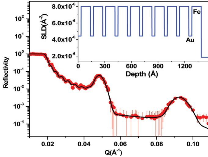
**Figure 1.** Unpolarized neutron reflectivity pattern from Fe/Au multilayer sample. Closed circles are experimental data whereas continuous line is fit to measurements. The inset shows the nuclear scattering length density (SLD)–depth profiling of multilayer.
