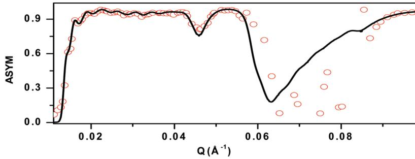
**Figure 3.** The spin asymmetry (ASYM) is plotted against  $Q$ . Open circles and continuous lines are the experimental data and corresponding fit to data, respectively.
