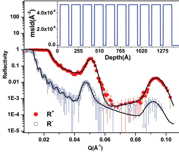
**Figure 2.** Polarized neutron reflectivity (PNR) pattern from Fe/Au multilayer sample. Closed and open circles are measured neutron reflectivity data for spin-up ( $R^+$ ) and spin-down ( $R^-$ ) neutrons, respectively, whereas the continuous lines are fit to measurements. Inset shows the magnetic scattering length density–depth profile of the sample.
