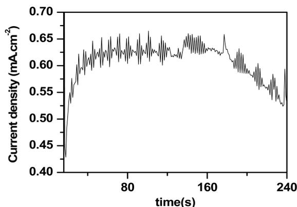
**Figure 1.** Current transient of Ni film recorded at  $0.5 V_{SCE}$  in  $0.095 M NaOH + 0.05 M H_2SO_4 + 0.05 M NaCl$  solution at  $pH = 3.0$ .
