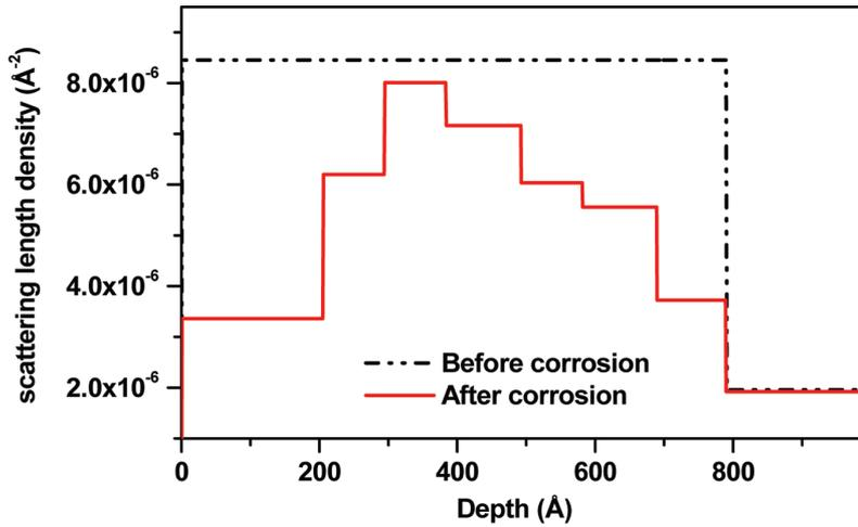
Figure 3. Scattering length density (SLD) profile of the sample extracted from fit to unpolarized neutron reflectivity measurements. Dash-dot-dot line is SLD profile of the as-deposited (before corrosion) sample whereas continuous line is SLD profile of the sample after corrosion.
