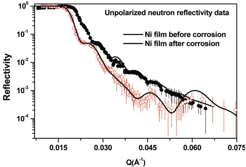
Figure 2. Specular unpolarized neutron reflectometry measurements on sample before (filled circles) and after (open circles) corrosion. Continuous lines are fit to measurements.
