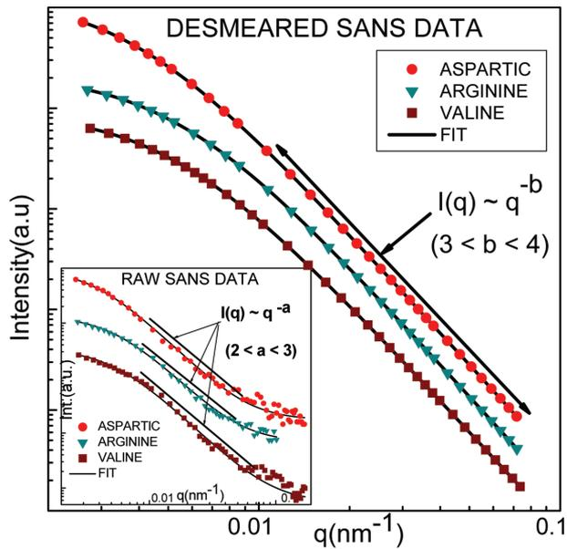
Figure 3. SANS profiles of sintered ceria pellets with fit.
