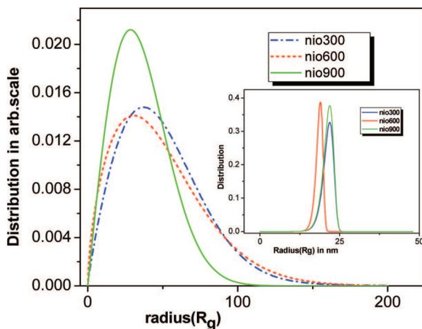
**Figure 4.** The larger length scale pore size distribution. Inset shows the smaller length scale pore size distribution.
