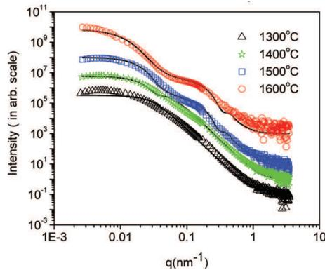
**Figure 4.** SANS profiles at three different sintering temperatures.
