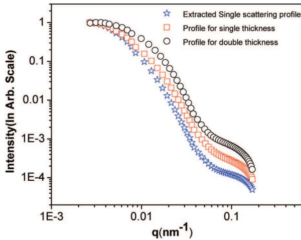
**Figure 1.** SANS profiles for two thicknesses and extracted single scattering profile for 1600°C sintered pellet.
