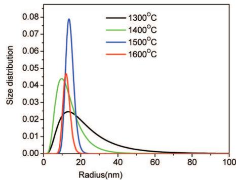
**Figure 5.** The pore size distribution for different sintering temperatures.
