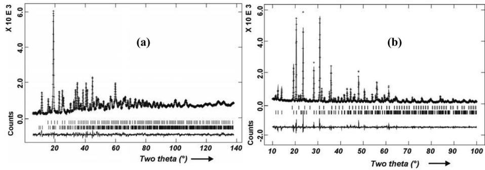
Figure 2. The typical Rietveld refinement plots for  $\text{Ca}_{0.5}\text{Ba}_{0.5}\text{Zr}_4\text{P}_6\text{O}_{24}$ . (a) ND and (b) XRD. Vertical marks between diffraction pattern and difference plot indicate Bragg positions for  $\text{ZrP}_2\text{O}_7$  (upper) and  $\text{Ca}_{0.5}\text{Ba}_{0.5}\text{Zr}_4\text{P}_6\text{O}_{24}$  (lower).
