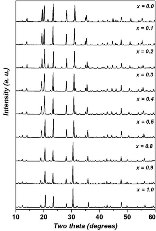
Figure 1. Powder XRD patterns of  $\text{Ca}_{1-x}\text{Ba}_x\text{Zr}_4\text{P}_6\text{O}_{24}$ .
