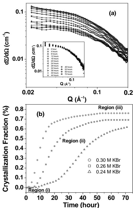
Figure 2. (a) Time-resolved SANS data of 1 wt% lysozyme with 0.24 M KBr and (b) measured crystallization fraction for 1 wt% lysozyme with three KBr concentrations.
