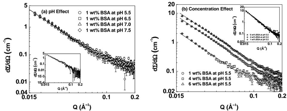
**Figure 6.** SANS data of protein gels of 1 wt% BSA prepared at (a) different pH and (b) different protein concentrations.
