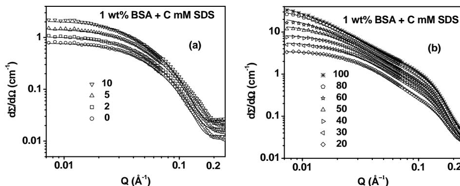
**Figure 3.** SANS data for 1 wt% BSA with varying SDS concentrations. (a) Low SDS concentrations and (b) high SDS concentrations.
