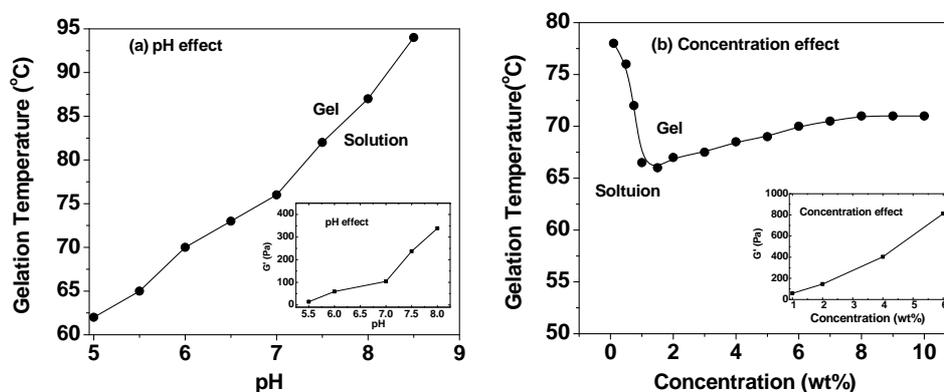
**Figure 5.** Temperature-induced phase diagram of protein gelation. (a) Effect of varying pH for 1 wt% BSA and (b) effect of concentration at constant pH of 5.5. Insets show the variation of storage modulus of the gels with pH or concentration.
