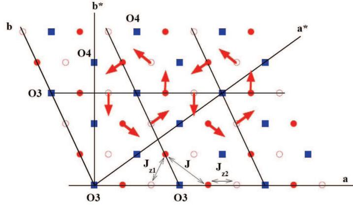
**Figure 1.** Schematic view of spin ordering [19] and atomic positions in  $\text{YMnO}_3$ . The squares depict oxygen O3 and O4 positions, while the circles indicate Mn position (filled and open symbols correspond respectively to the  $z = 0$  and the  $z = 1/2$  plane). The magnetic and chemical unit cells are identical with lattice parameters  $a = 6.14 \text{ \AA}$  and  $c = 11.39 \text{ \AA}$ .
