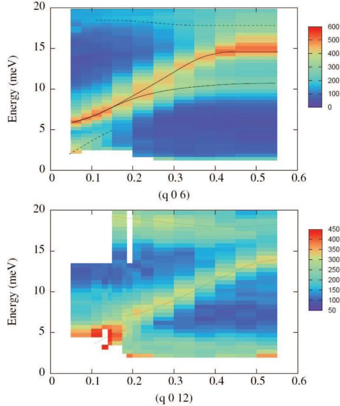
**Figure 3.** Colour mappings of the neutron intensity obtained as a function of energy transfer and wave vector along  $a^*$ . The data were taken at  $T = 18$  K around  $(0, 0, 6)$  Bragg position (upper panel) and around  $(0, 0, 12)$  (lower panel). Solid and dashed lines are guides to the eyes.
