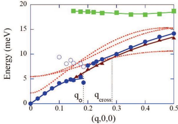
**Figure 4.** Phonon dispersions obtained at 200 K (triangles) and 18 K (circles). Closed and open symbols correspond to large and small intensities respectively. The squares correspond to the optic phonon mode. Red dotted lines are calculated spin wave dispersions. The gap in the phonon dispersion opens at  $q_0$ . Crossing of the 200 K phonon dispersion with the spin wave mode 3 arises at  $q_{\text{cross}} \sim 0.3$ .
