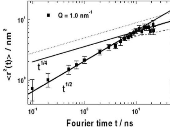
**Figure 1.** Time-dependent mean square displacement of a PEP segment in the melt at 492 K. The solid line indicates the prediction of the Rouse model [6]. The slowing down at longer times is an indication of a cross-over to local reptation (see ref. [6]).
