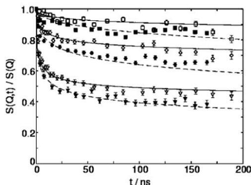
**Figure 4.** Dynamic structure factor of a centre-labelled 25 kg mol<sup>-1</sup> PE chain (filled symbols) compared to a fully labelled chain (open symbols) of the same overall molecular weight.  $Q$  values (in nm<sup>-1</sup>): 0.5 (squares), 0.77 (diamonds), 0.96 (circles), 1.15 (triangles). Lines: for centre-labelled chain, pure reptation model (eq. (2)); for fully labelled 25 kg mol<sup>-1</sup> chain (dashed) CLF was considered [11,17].
