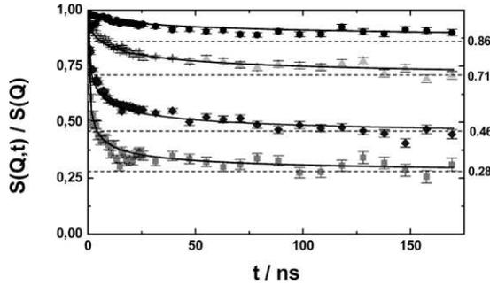
**Figure 2.** The dynamic structure factor from a  $M_w = 36 \text{ kg mol}^{-1}$  PE melt at 509 K as a function of time. The solid lines are a fit with the reptation model (eq. (2)). The  $Q$  values from the top are  $Q = 0.5, 0.77, 1.15$  and  $1.45 \text{ nm}^{-1}$ . The horizontal dashed lines display the prediction of the Debye–Waller factor estimate for the confinement size (see text).
