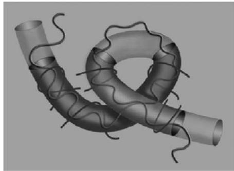
**Figure 3.** Schematic presentation of the CLF and CR mechanisms: chain end fluctuations lead to a shortening of the effective tube length, while the dissolving of entanglements allow chain motions beyond the initial tube constraints [12].
