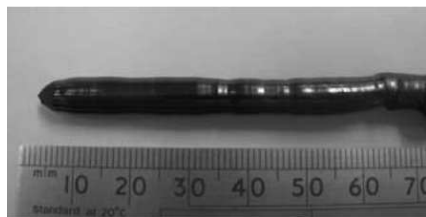
Figure 5. As grown crystal boule of \text{Ni}_3\text{V}_2\text{O}_8 .
