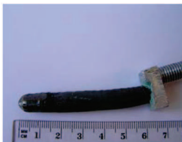
Figure 2. Large single crystal of magnetite ( \sim 4.5 cc) used in a neutron scattering experiment at ISIS.
