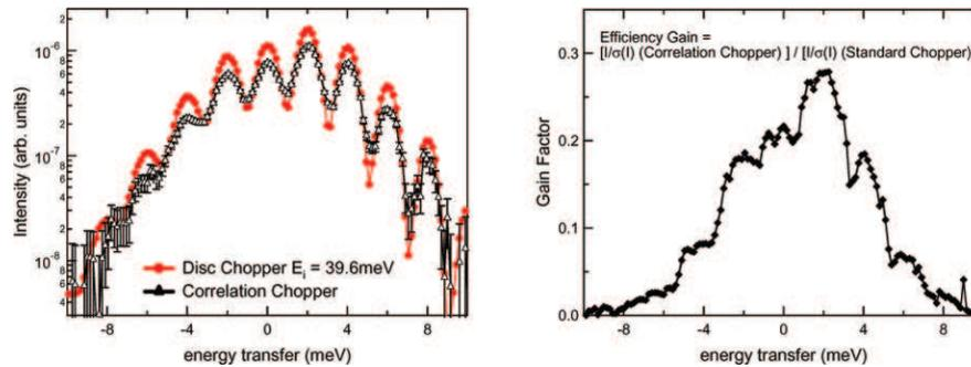
**Figure 3.** Comparison of a single spectrum with fixed incident energy extracted from the cross-correlated data with the spectrum measured with a traditional single-aperture chopper (left) and corresponding gain in efficiency of the cross-correlation (right).
