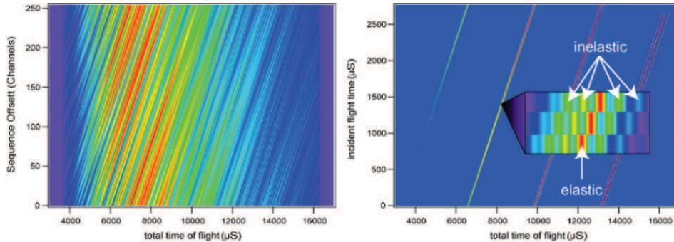
**Figure 2.** Intensity measured by the detector as a function of total time-of-flight and correlation sequence phase-offset and the corresponding cross-correlated data obtained for the full experiment simulations using a harmonic oscillator sample.
