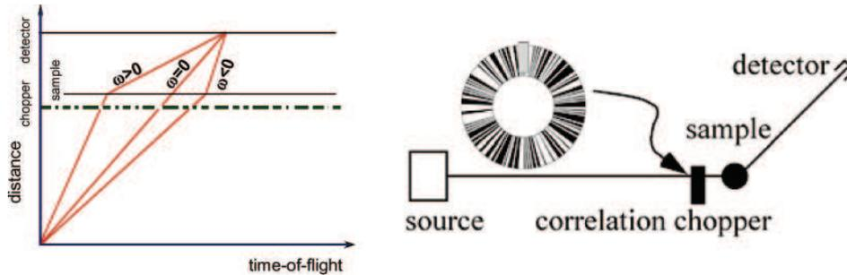
**Figure 1.** Illustration of the intensity measured with the cross-correlation technique at fixed total time-of-flight (left) and schematic of the simplified instrument used for the simulations (right).
