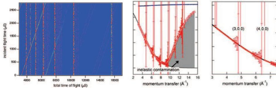
**Figure 4.** Full experiment simulation using a perfect coherent scatterer and including Bragg peaks. The middle panel shows the elastic scattering extracted from the cross-correlated data in red and the total scattering  $S(Q)$  in blue. The right panel shows an enlarged region from the middle panel around the (3,0,0) and (4,0,0) Bragg peaks.
